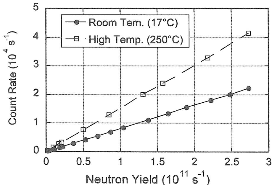
Fig. 7.1-3 Pulse count rates of the micro-fission chamber as a function of the neutron yields.
