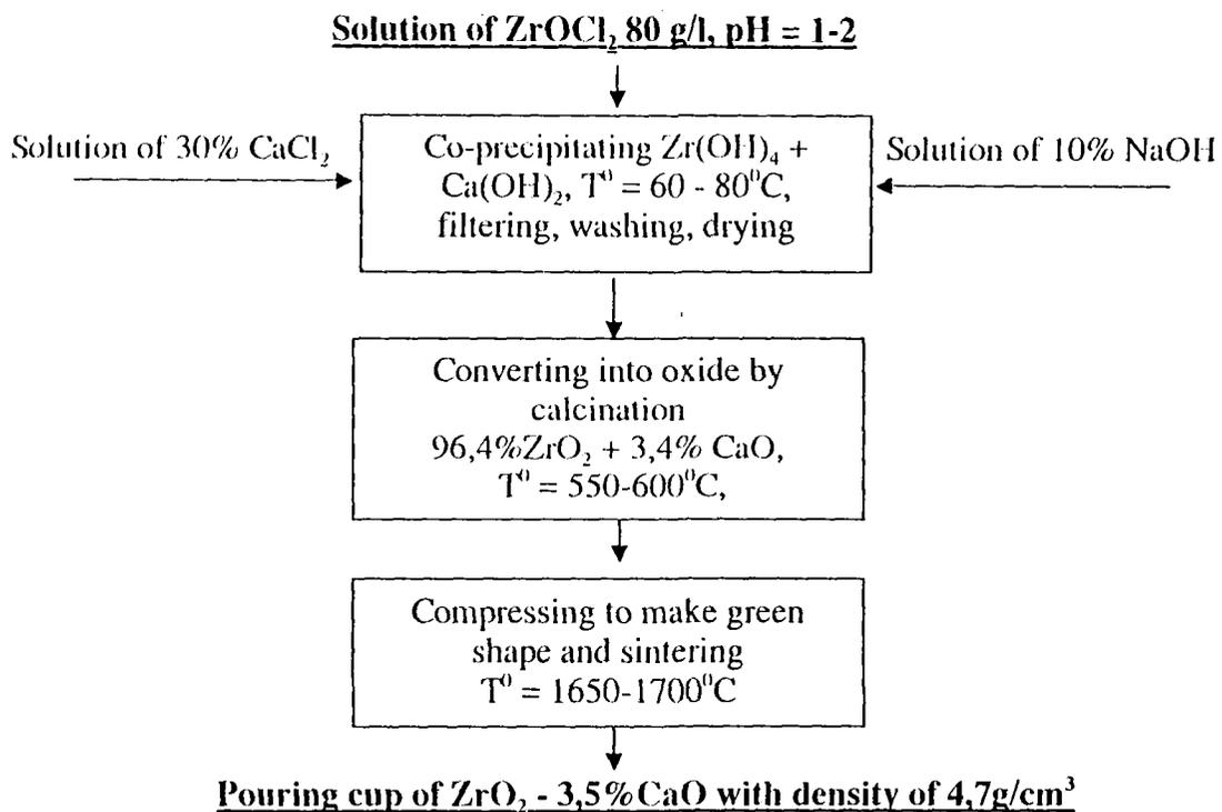
**Figure 1:** Diagram of preparation of stabilized calcium zirconium oxide ceramic powder by co-precipitation and testing production of pouring cup by stabilized zirconium dioxide.
