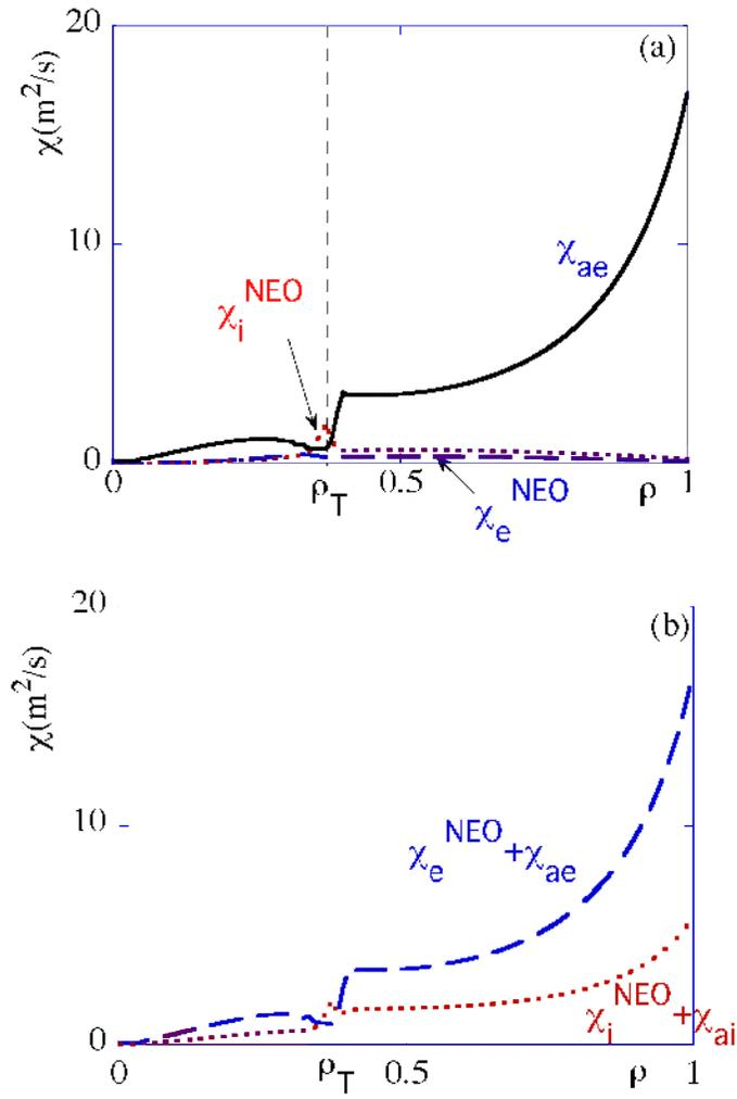
**Figure 2.** Radial profiles of the anomalous and neoclassical diffusivities in figure 2(a). In figure 2(b), the sum of the anomalous and neoclassical diffusivities is shown. These figures correspond to the case of figure 1.
