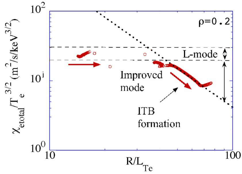
**Figure 4.** Normalized heat diffusivity calculated as a function of  $R/L_{T_e}$  at  $\rho = 0.2$ . The arrow indicates the temporal direction. The dotted line represents the relation  $\chi_{\text{etotal}}/\Gamma_e^{3/2} \propto (R/L_{T_e})^{-2.2}$ .
