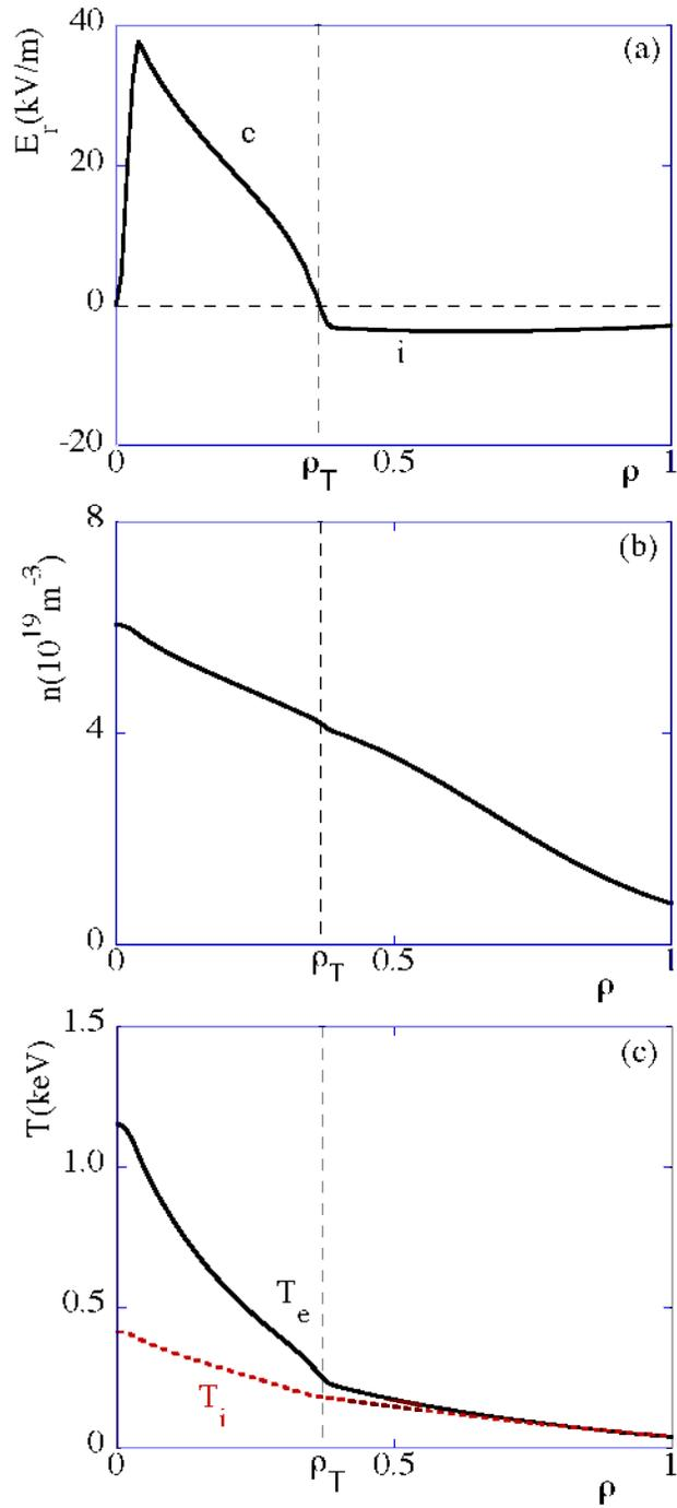
**Figure 1.** (a) Radial dependence of the electric field (full curve). (b) radial profile of the density. (c) profiles of the temperatures of ions and electrons. The absorbed power of electrons is 100kW and that of ions is 0kW, respectively. The coefficient  $S_0$  of the particle source is  $5 \times 10^{22} \text{m}^{-3} \text{s}^{-1}$ .
