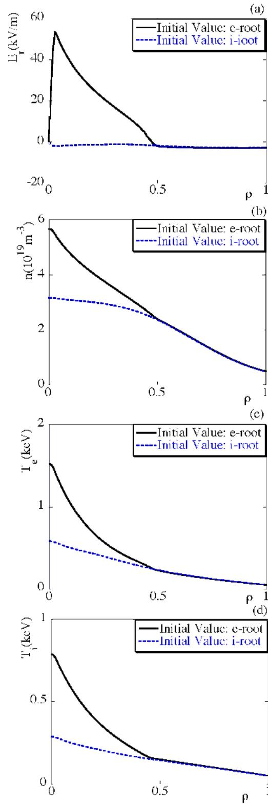
**Figure 3.** (a) Radial dependence of the electric field. (b) Radial profile of the density. (c) profiles of the electron temperature and (d) profiles of the ion temperature. The full curve and dotted curve show the steady state from the initial condition of the electron root and ion root, respectively. The absorbed power of electrons is 100kW and that of ions is 10kW, respectively. The coefficient  $S_0$  of the particle source is  $7 \times 10^{22} \text{ m}^{-3} \text{ s}^{-1}$ .
