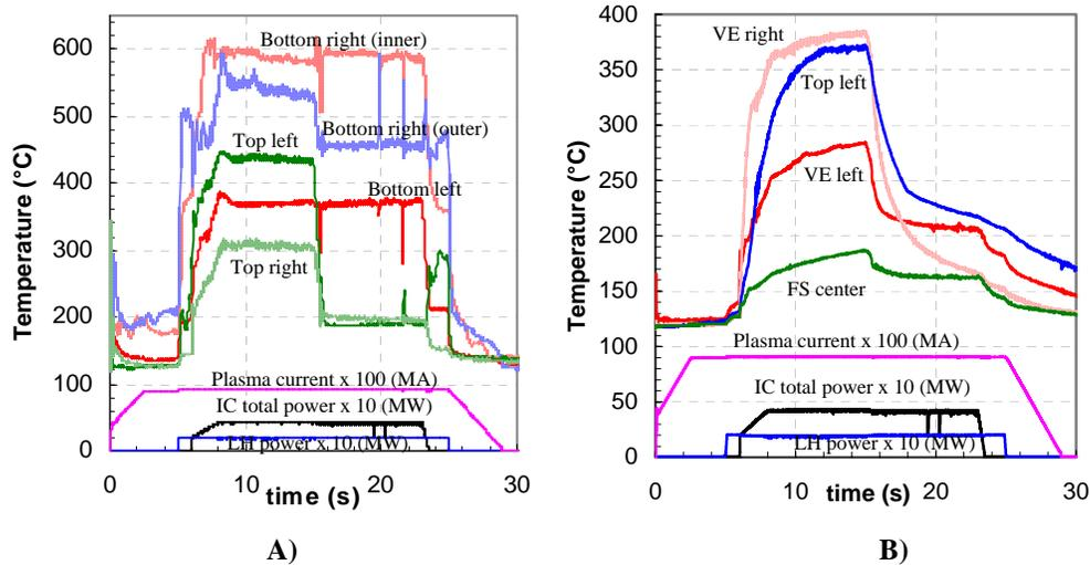
**FIGURE 2. EFFECT OF IC TOTAL/PRIVATE/LH POWER A) Guard limiters time traces B) Faraday screen time traces (IC launcher switched off at 15 s at constant total IC power)**
