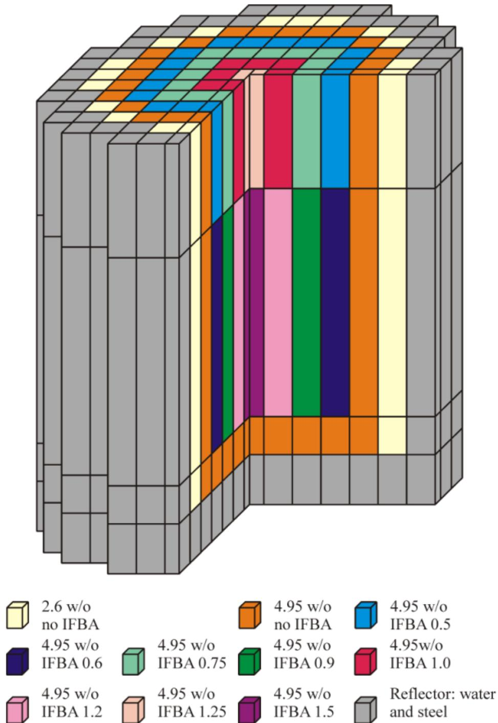
Figure 3: 3D Axial and radial distribution of IFBA
