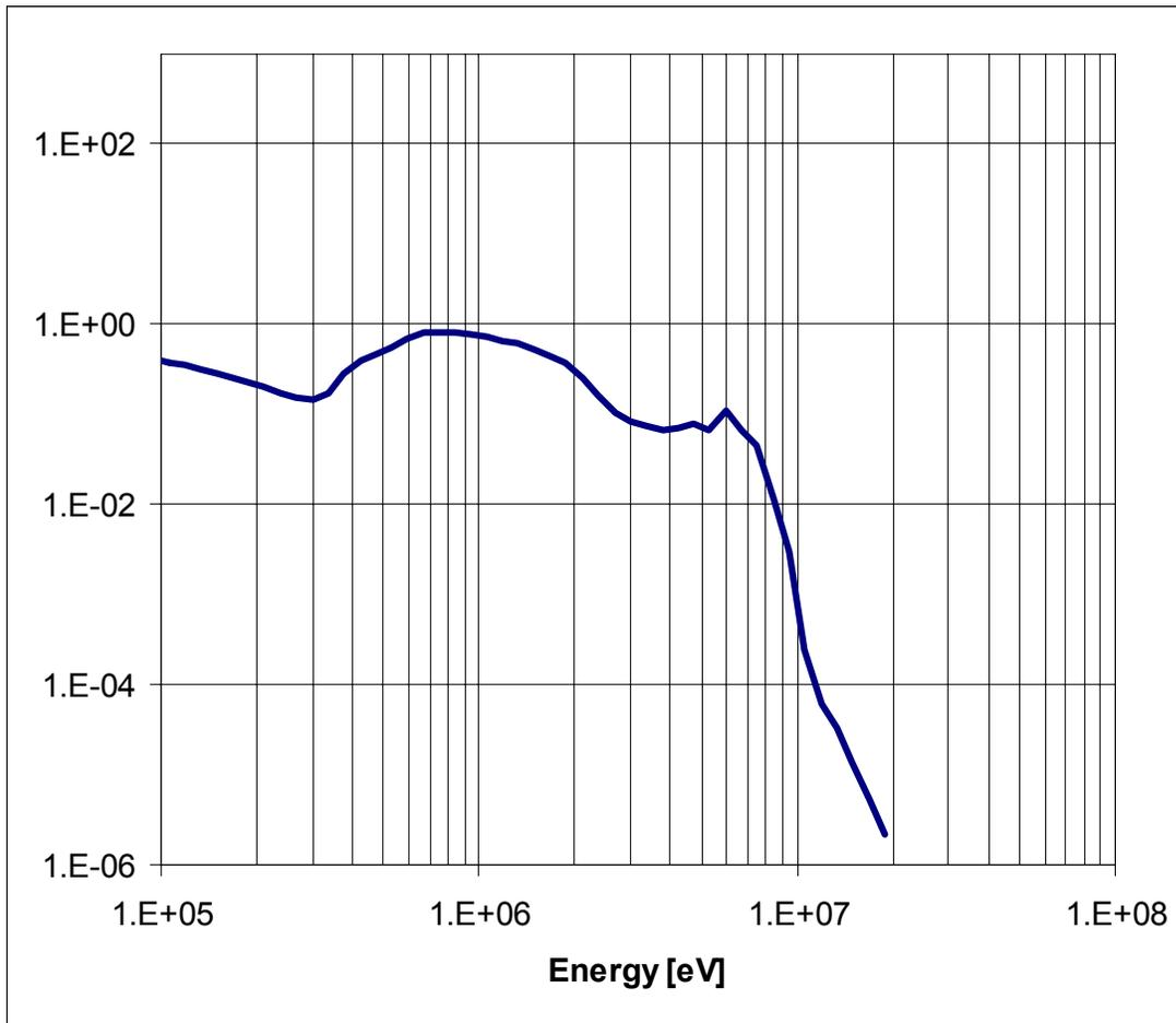
Figure 2. Fast neutron spectrum at the standard irradiation position in the exposure room at reactor power of 250kW.
