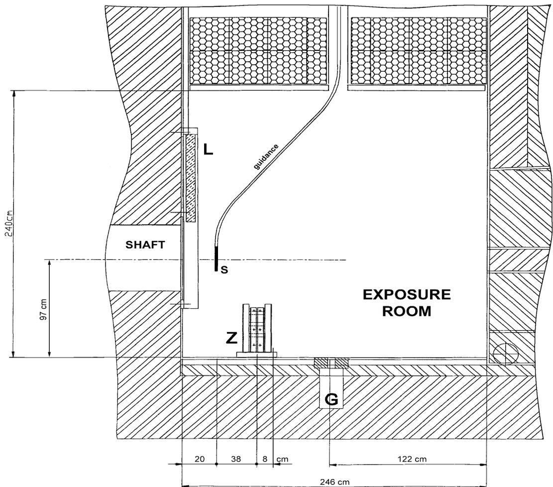
Figure 1. Simplified vertical cross-section through the dry cell.
