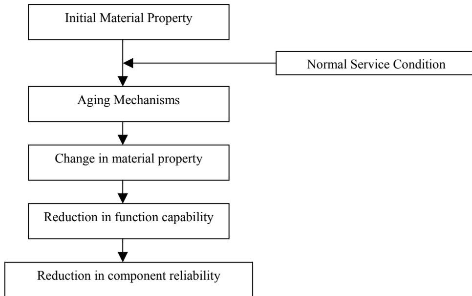
Figure 2.1. Impact of service conditions on material degradation and component reliability
