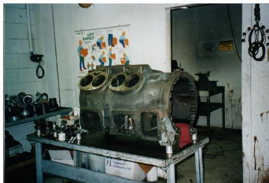
Figure 5: Refrigeration Compressor Maintenance
