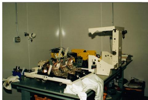
Figure 3: Maintenance of GE AK-75 Series Breaker
