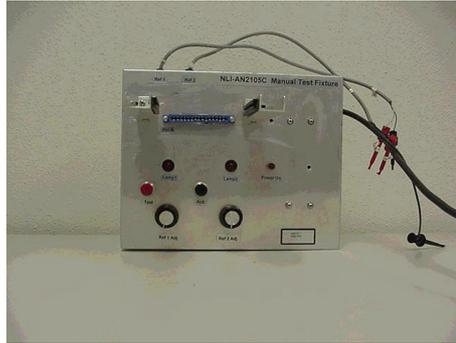
Figure 2: In many cases, in order to simulate the board's true safety function a test box as shown above is used to simulate the "host" that the board would normally be installed in.
