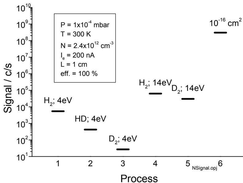
Figure 4: Expected signal from detection method based on DEA to  $H_2$ , HD and  $D_2$ . Cross sections for higher vibrational states in all isotopomer reach  $10^{-16} \text{ cm}^2$  that is also shown.
