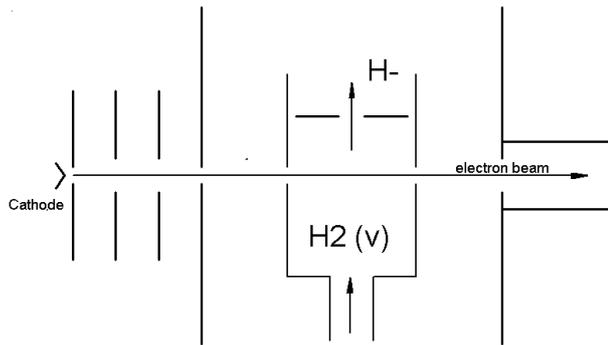
Figure 1: Schematic representation of hydrogen ro-vibrational diagnostics based on the dissociative electron attachment.
