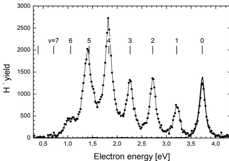
Figure 2:  $H^-$  yield as a function of electron beam energy for the cold ( $v=0$ ) gas (full line) and for vibrationally hot gas (dot and line).
