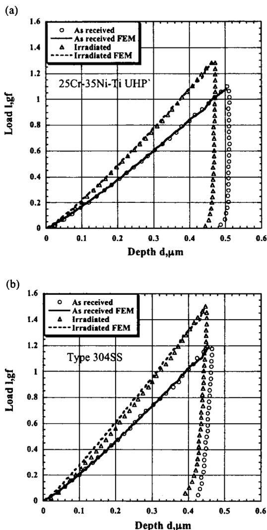
Fig.5 L-D curves measured using the conical indenter, and the calculated results by the inverse analysis
