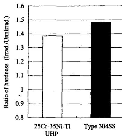
Fig.4 Relative ratio of hardness for specimens irradiated 50dpa by triple ion beams to it of original specimens at 278K
