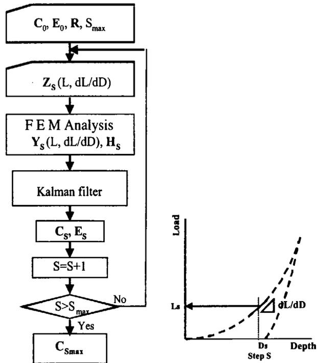
Fig.2 Flow chart for identification of material constants
