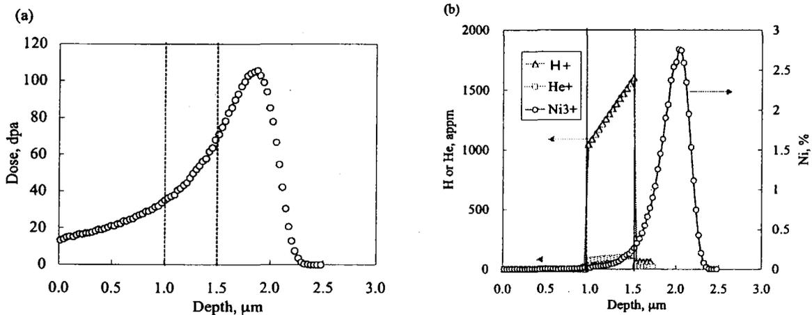
Fig.1 Depth profiles of (a) displacement damage by nickel and (b) nickel, hydrogen and helium concentrations in the specimen irradiated by triple beams
