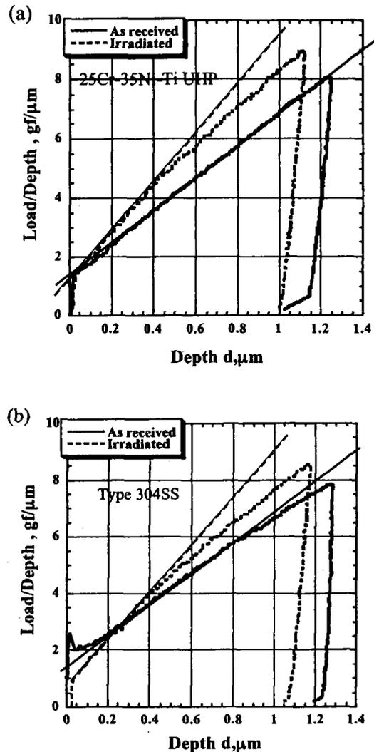
Fig.3 load/depth-depth (L/D-D) curves of 25Cr-35Ni-Ti UHP and type 304
