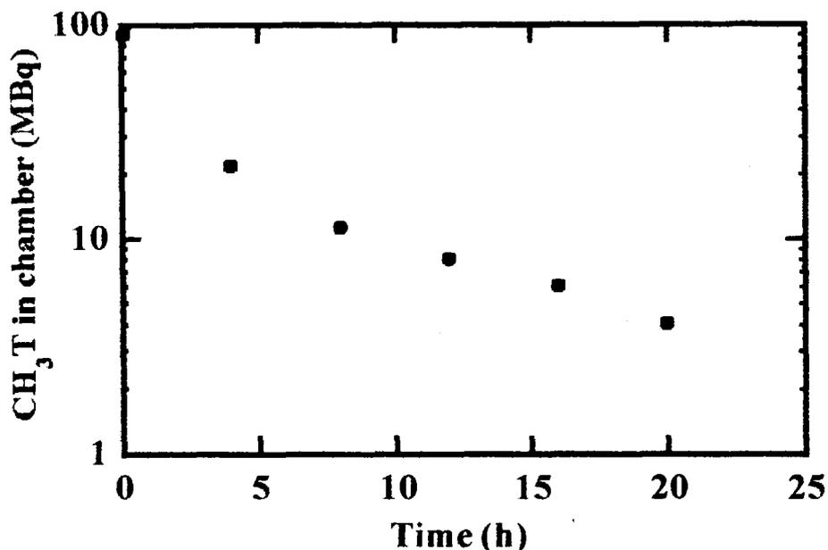
Fig. 1. Time course of tritiated methane ( $\text{CH}_3\text{T}$ ) in the experimental chamber. (The plots were average in duplicate.)
