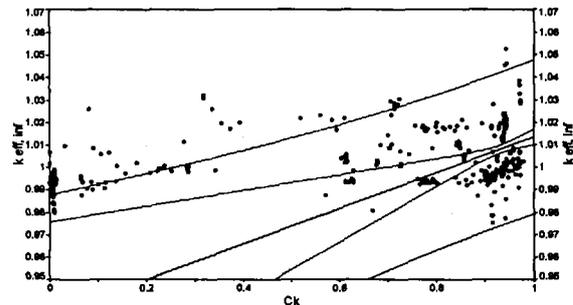
**Fig. 2** Infinite array of TRUPACT-IIs with 55-gallon drums,  $k_{eff, inf} = 0.9340 + 0.0797c_k$  (1.0137) with 99% confidence intervals.
