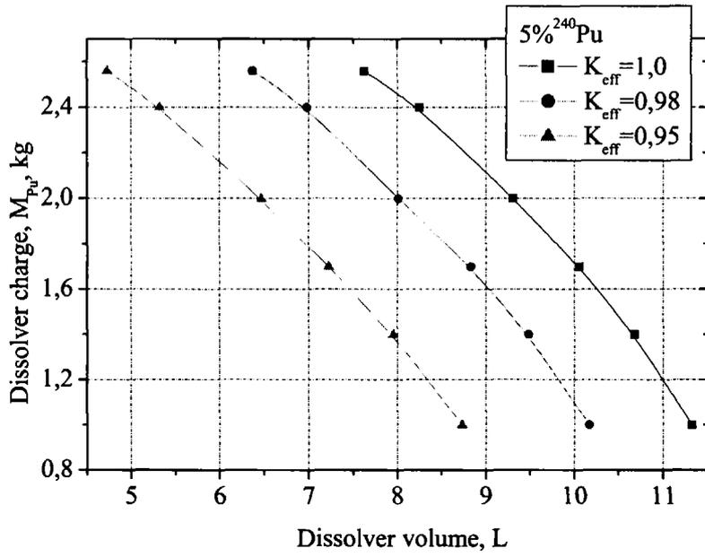
Fig.4. Dissolver charge as a function of its volume at 5% <sup>240</sup>Pu.
