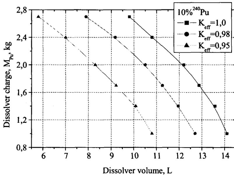
Fig.5. Dissolver charge as a function of its volume at 10% <sup>240</sup>Pu.
