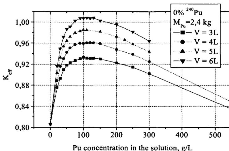
Fig.1.  $K_{eff}$  of the dissolver as a function of Pu concentration in the solution and dissolver volume at 0%  $^{240}\text{Pu}$ .
