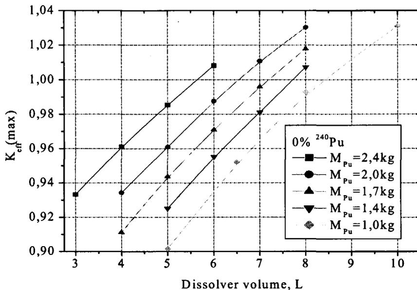
Fig.2. The maximum  $K_{eff}$  value as a function of dissolver volume and its charge at 0%  $^{240}\text{Pu}$ .
