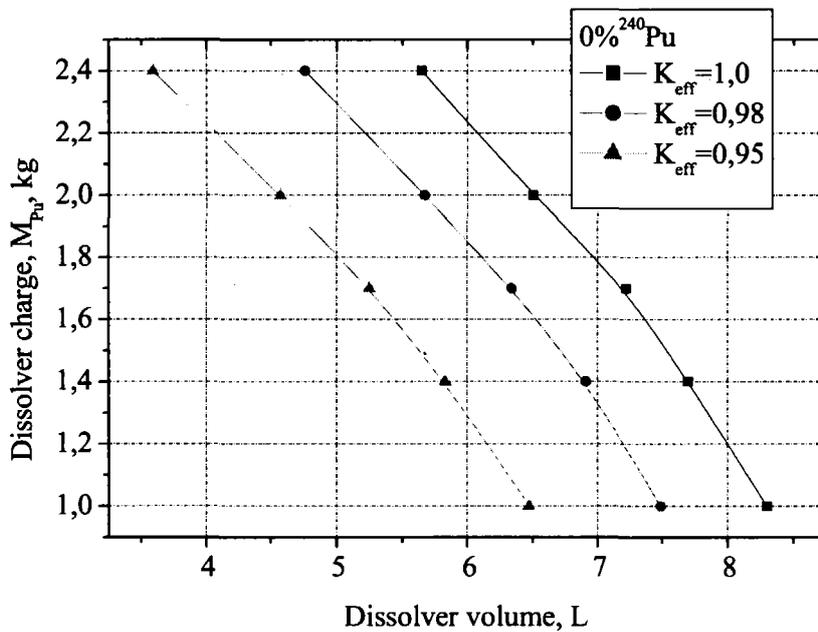
Fig.3. Dissolver charge as a function of its volume at 0%  $^{240}\text{Pu}$ .
