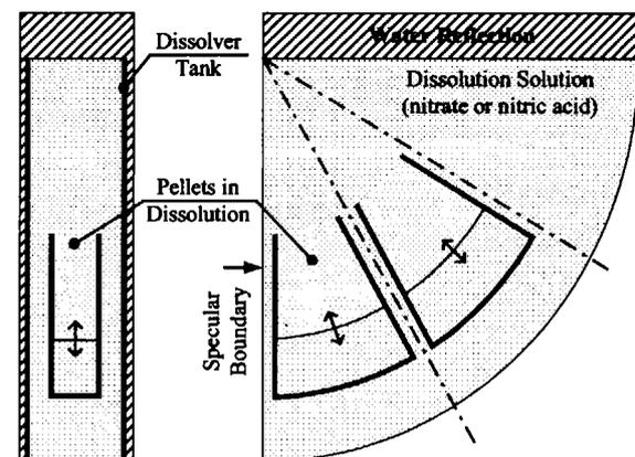
**Fig.1** Schema of the rotary dissolver modeling
