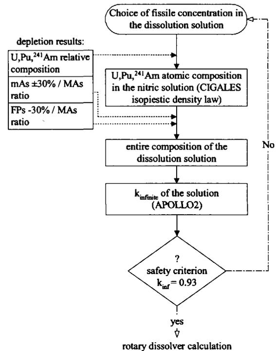
**Fig.2** Calculation diagram of the nitrate solution’s study
