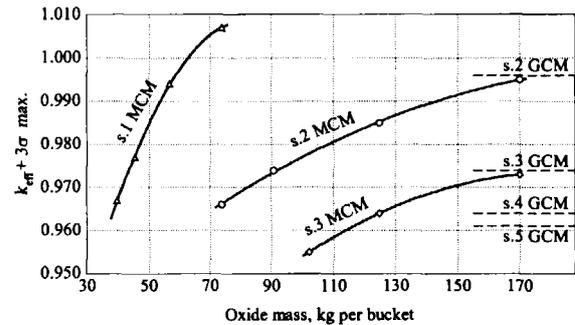
**Fig.4** maximal  $k_{eff} + 3\sigma$  values (whatever pellets' radius and moderator-to-fuel ratio are) for MOX pellets in dissolution into the rotary dissolver. "s.i" is relative to the BUC sequence number *i*. MCM and GCM respectively mean "mass control mode" and "geometry control mode".
