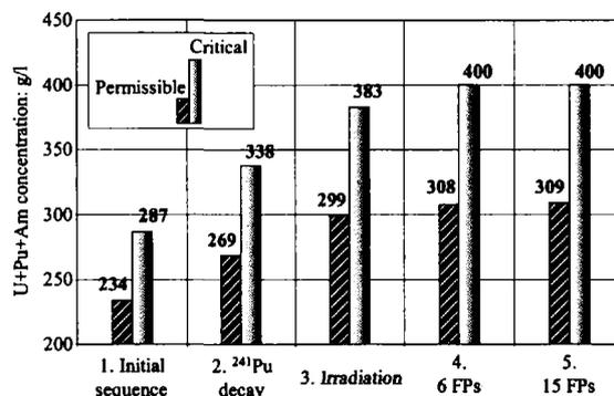
**Fig.3** Permissible and critical fissile concentration in the nitrate solution for each BUC sequence.
