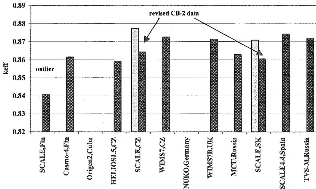
Fig. 2 KENO VI keff sensitivity calculations for VVER conceptual cask with 3.6% fuel, 30 MWd/kg uniform burnup, 5y cooling time (the mean of the original data: 0.864,  $\sigma=1.1\%$ , the mean of the data without the outlier: 0.867,  $\sigma=0.7\%$ )
