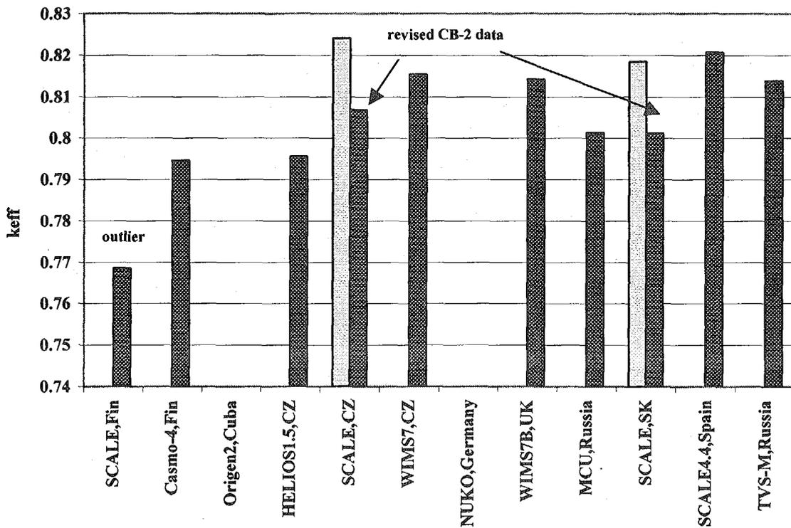
Fig. 4 KENO VI keff sensitivity calculations for VVER conceptual cask with 3.6% fuel, 40 MWd/kg uniform burnup, 5y cooling time (the mean of the original data: 0.803,  $\sigma=1.9\%$ , the mean of the data without the outlier: 0.807,  $\sigma=1.2\%$ )
