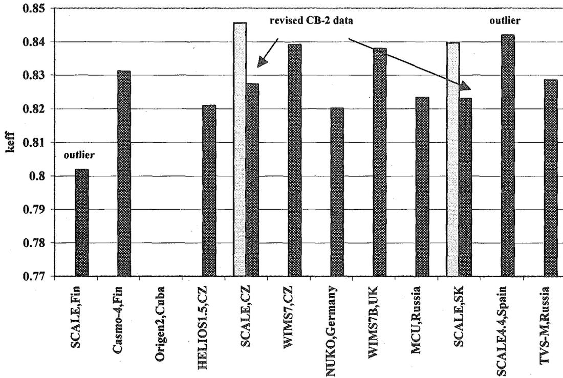
Fig. 3 KENO VI keff sensitivity calculations for VVER conceptual cask with 3.6% fuel, 40 MWd/kg uniform burnup, 1y cooling time (the mean of the original data: 0.827,  $\sigma=1.4\%$ , the mean of the data without the outliers: 0.828,  $\sigma=0.8\%$ )
