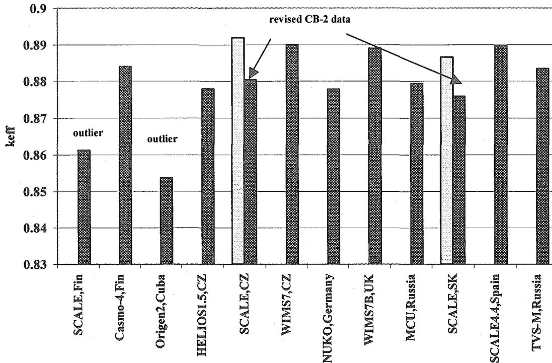
Fig. 1 KENO VI keff sensitivity calculations for VVER conceptual cask with 3.6% fuel, 30 MWd/kg uniform burnup, 1y cooling time (the mean of the original data: 0.879,  $\sigma=1.3\%$ , the mean of the data without the outliers: 0.883,  $\sigma=0.6\%$ )
