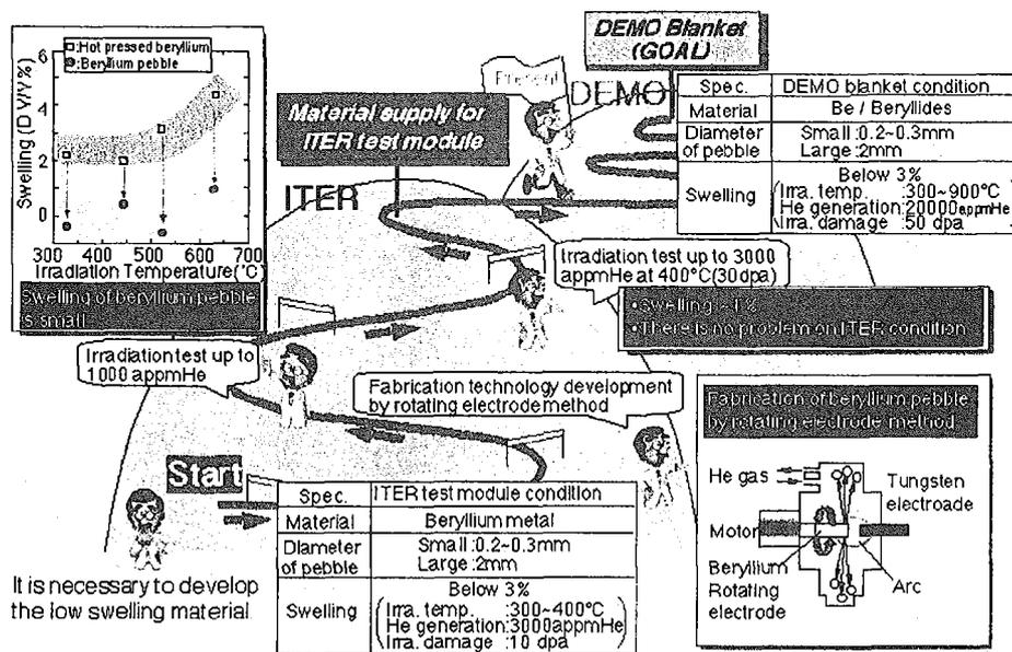
Fig.1 Development of neutron multiplier for DEMO blanket
