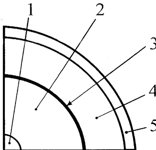
FIGURE 2. Post-irradiation structure of a target sector: (1) deposition zone; (2) zone of Be-sputtering and sputtered atoms re-deposition; (3) dark zone; (4) re-deposition zone; (5) exterior sector ring shielded by a screen during ion bombardment.
