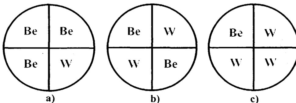
FIGURE 1. Compound sector targets with different Be to W area ratios.
