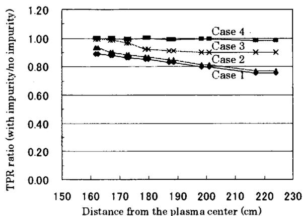
Figure 6. Effect of impurities on fusion DEMO-reactor blanket.
