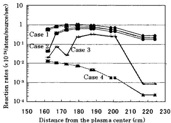
Figure 5. TPR distributions in fusion DEMO-reactor blanket.
