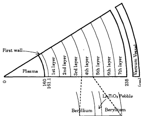
Figure 4. Calculation geometry of fusion DEMO-reactor blanket.
