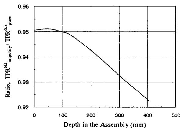
Figure 2. Effect of impurity as a function of depth in beryllium assembly.
