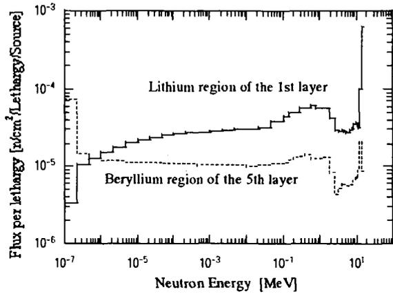
Figure 7. Neutron spectra in fusion DEMO-reactor blanket.
