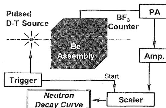
Figure 3. Pulsed neutron decay experiment system.
