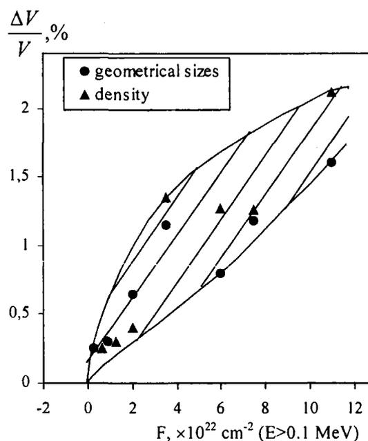
Figure 4. Dose dependence of swelling for the TE-56 beryllium grade irradiated at 70°C
