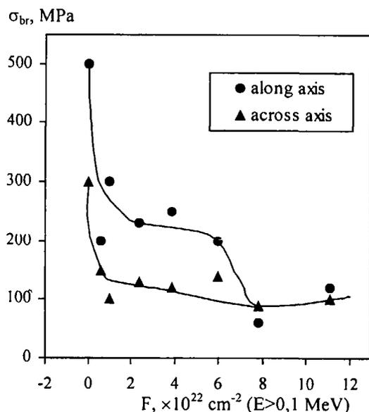
Figure 5. Dose dependence of brittle strength ( $\sigma_{br}$ ) for the irradiated TE-56 beryllium grade ( $T_{irr}=70^{\circ}\text{C}$ ,  $T_{test}=20^{\circ}\text{C}$ ) according to mechanical tensile tests
