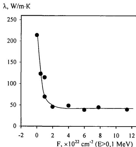
Figure 6. Dose dependence of thermal conductivity for the TE-56 beryllium grade, along the axis at  $T_{irr}=T_{test}=70^{\circ}\text{C}$
