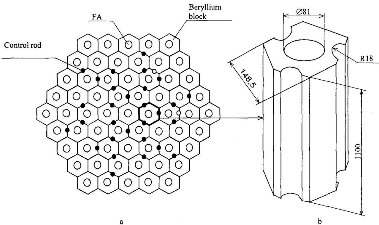
Figure 2. The MIR reactor core:
