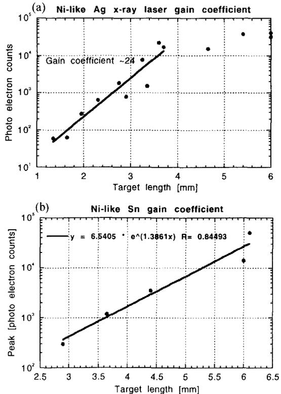
**Fig.3 Output intensity of x-ray lasers vs. target length. The gain coefficients were determined by fitting the Linford formula to those data in the exponential region, to be 23cm<sup>-1</sup> for Ag (a) and 14cm<sup>-1</sup> for Sn (b).**
