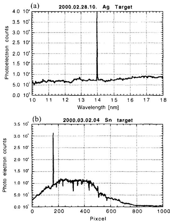
**Fig2 Time integrated axial spectrums. Figs. 2 (a) and (b) are the spectrum of the x-ray from Ag and Sn targets, respectively.**
