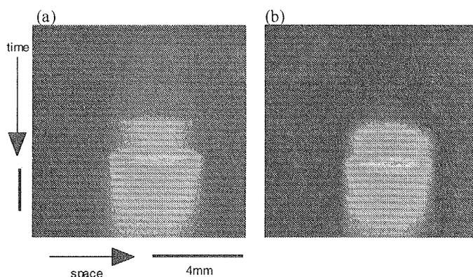
**Fig.4 Temporal image of x-ray laser plasmas. Figs. 4(a) and (b) are the data with 1.5ps pre-pulse and 600ps pre-pulse with Titanium targets. The Fig. 4(b) shows the evidence of nonlinear scattering from a quarter critical density and self-focusing.**
