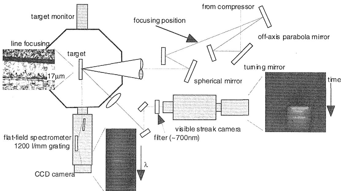
**Fig.1** Experimental setup for the x-ray laser generation. The laser pulses were focused onto slab targets with a combination of an off-axis parabola mirror and a spherical mirror. The x-ray spectrum was measured with a flat-field spectrometer. The scattered emission from the gain plasma was measured with a filtered visible streak camera.
