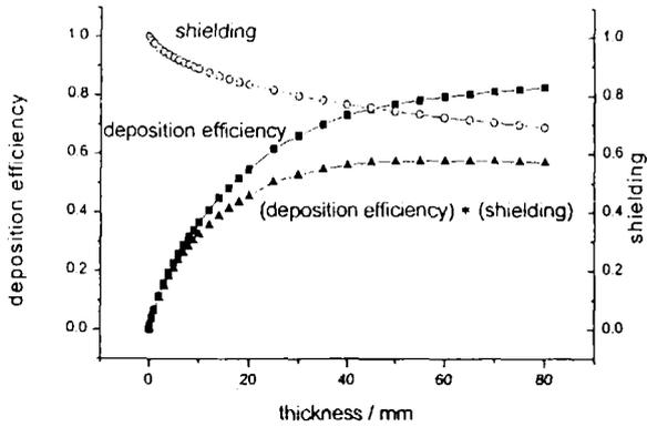
Fig. 3 Energy deposition efficiency and neutron shielding effect. (thickness=60mm, energy deposition efficiency=79.6%, neutron shielding effect=72.3%, total efficiency=57.5%)
