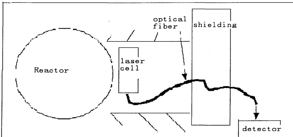
Fig.1 Scheme of nuclear pumped laser set-up
