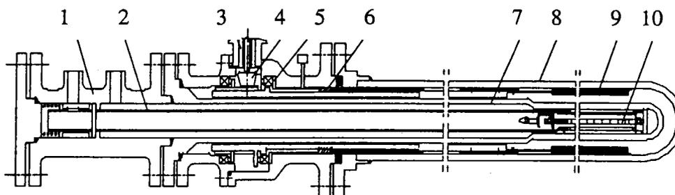
Fig.2-1 Configuration of the in-pile power ramp test facility<sup>(3)</sup>
