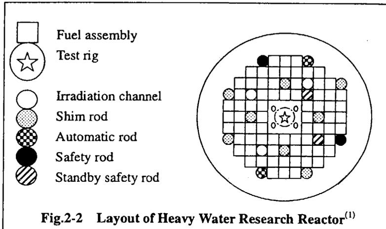
Fig.2-2 Layout of Heavy Water Research Reactor<sup>(1)</sup>
