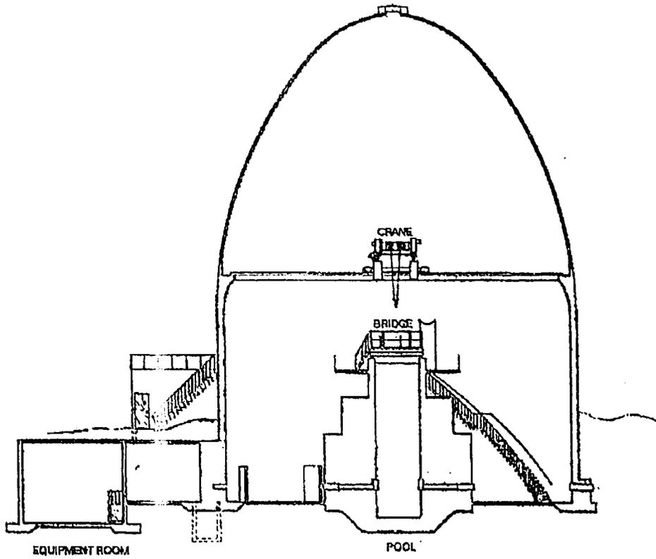
Figure 1. Transverse section of the reactor building.
