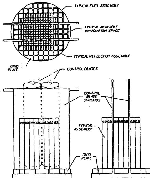
Figure 5. Three views of the new grid plate with fuel and reflector assemblies and control blade
