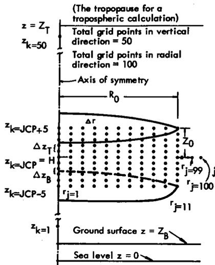
Figure 4. Grid system for the numerical diffusion model.
