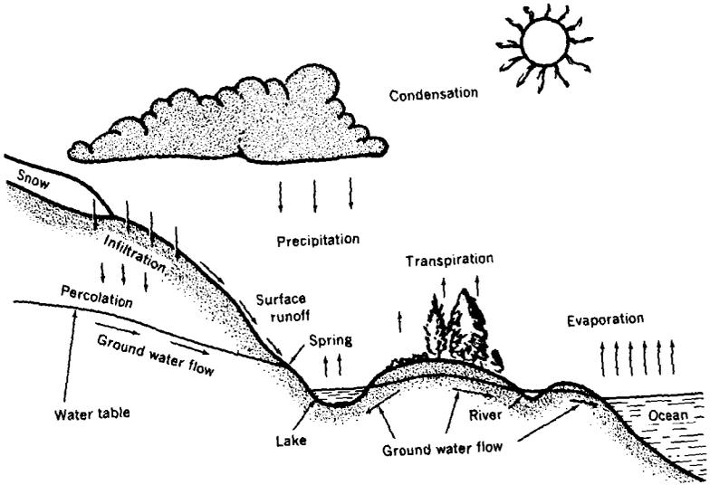
Figure 1. The hydrologic cycle.
