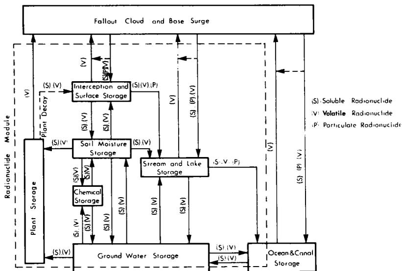
Figure 3. Diagrammatic Model of Radionuclide Transport By Water
