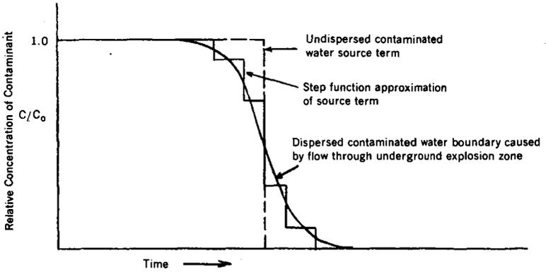
Figure 7. Source Term for Flow from Underground
