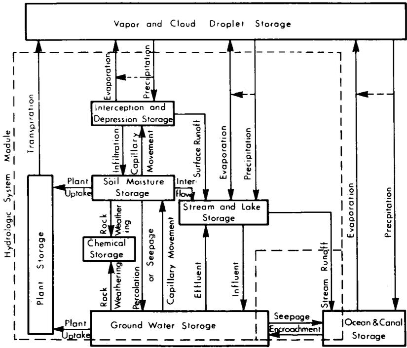
Figure 2. Diagrammatic Model of the Hydrologic Cycle.
