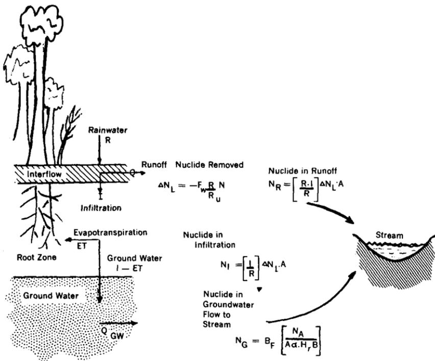
Figure 9. Schematic Diagram of the Fallout-Zone Redistribution
