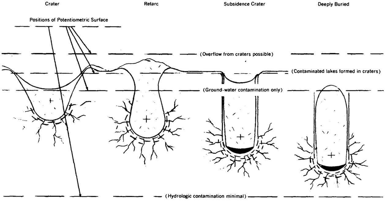
Figure 4. Relationship of Detonation Effects to Potentiometric Surface
