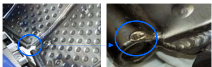
Vessel protection panel SS melting due to ripple trapped ions, 3 MW/m 2 power density. Water leak occurrence : November 2003
