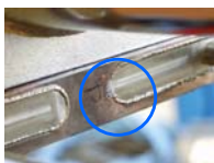
endoscope ripple protections micro leak July 2003
