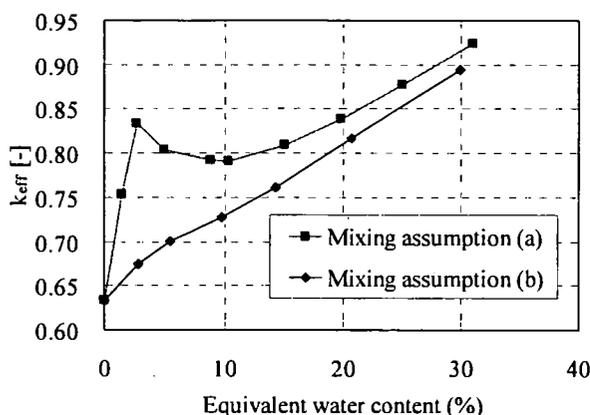
Fig.5  $k_{\text{eff}}$  vs. equivalent water content for 640kg MOX(18%Pu content,  $5.5\text{g/cm}^3$ ), zinc stearate ( $0.3\text{g/cm}^3$ ).
