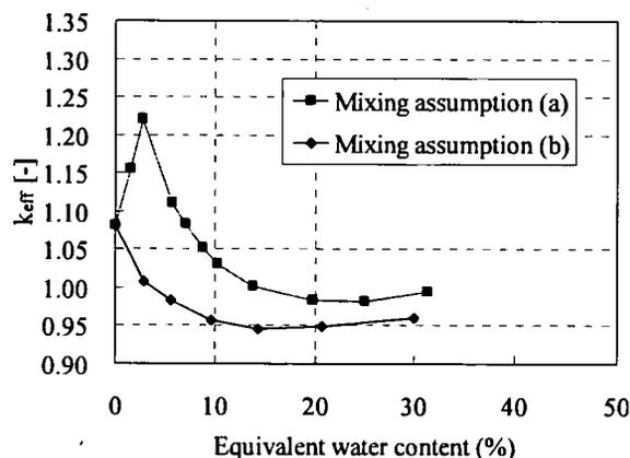
Fig.3  $k_{\text{eff}}$  vs. equivalent water content for 640kg MOX(50%Pu content,  $5.5\text{g/cm}^3$ ), zinc stearate ( $0.3\text{g/cm}^3$ ).
