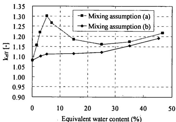
Fig.4  $k_{\text{eff}}$  vs. equivalent water content for 640kg MOX(50%Pu content,  $5.5\text{g/cm}^3$ ), zinc stearate ( $0.6\text{g/cm}^3$ ).
