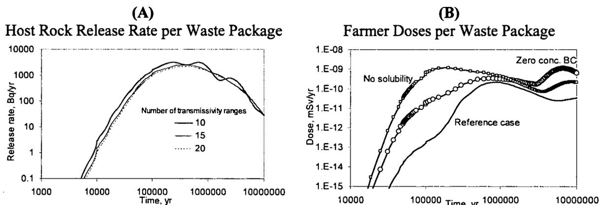
**Figure 3.** (A) Host rock release rates per waste package as a function of the transmissivity domain stratification. (B) Doses to farmer receptor group under three cases: reference case, no solubility constraints in the buffer material, and zero concentration boundary condition at the end of the buffer material.
