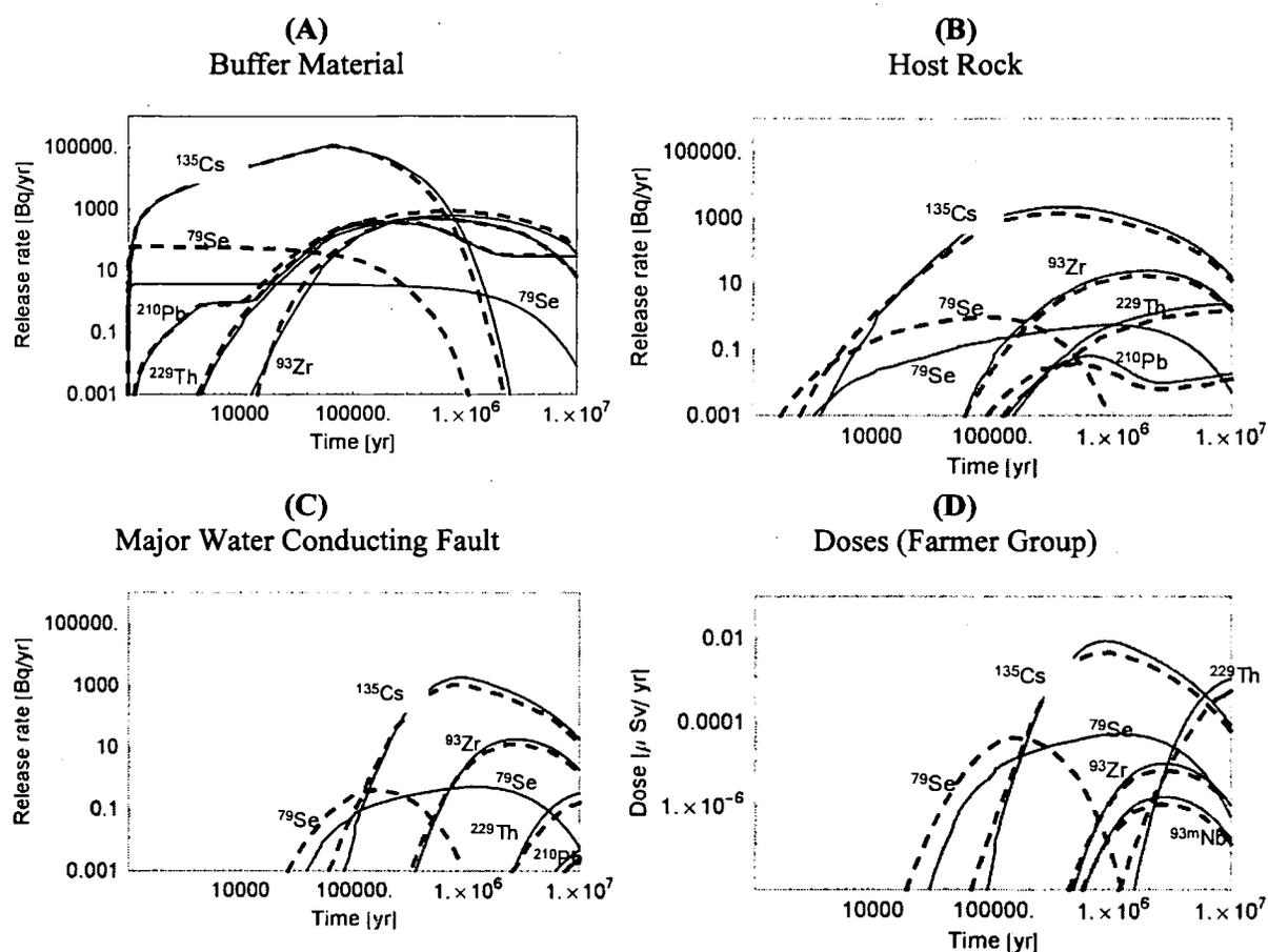
**Figure 2.** Radionuclide release rates per waste package at various points in the system: (A) away from the buffer material, (B) away from the host rock, (C) away from the MWCF into the biosphere. (D) Doses to the farmer receptor group from 40,000 failed waste packages.
