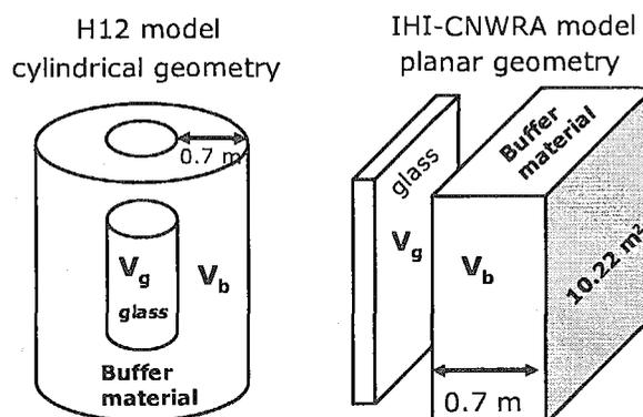
**Figure 1.** Cylindrical geometry (H12 model) and planar geometry (IHI–CNWRA model) adopted to describe the buffer material.
