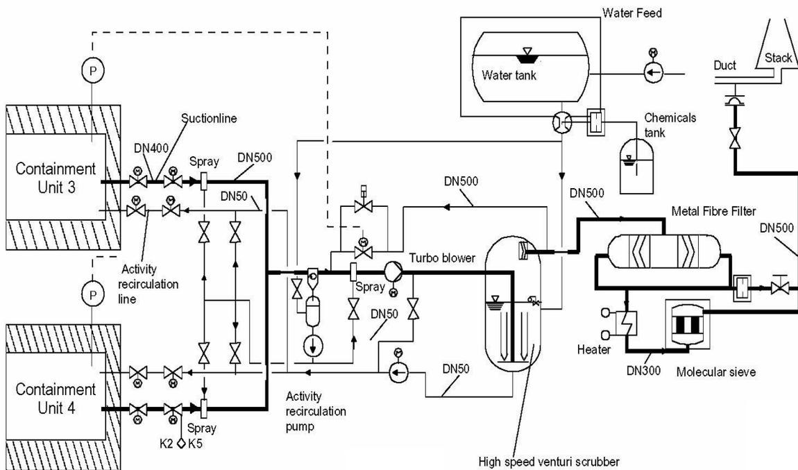
The connection of the Containment Leakage Control and Venting System to the containment is done by containment isolation flaps and suction lines with integrated spray nozzles, arranged in the Reactor Building. The main system components are installed in a special compartments inside the reactor building on an elevation which is even to the containment bottom elevation.
