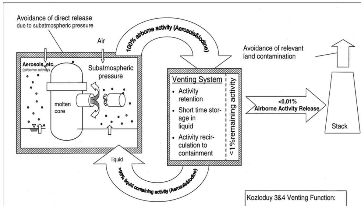
During a hypothetical event of a beyond design basis accident with core melting, the pressure in the containment will increase. This increased pressure will cause uncontrolled release of radioactive products to the environment through the leaks of the accident localization system.
