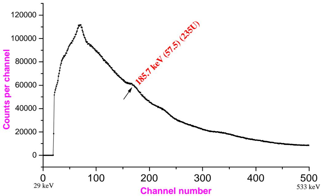
**Figure 2. Gamma ray spectrum of Uranium (66 mg/l) on NaI(Tl) detector**
