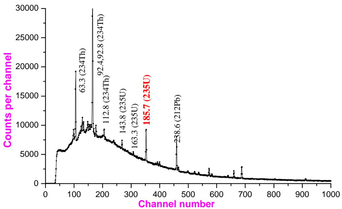
**Figure 3. Gamma ray spectrum of Uranium (10mg/l) on 10% HPGe**
