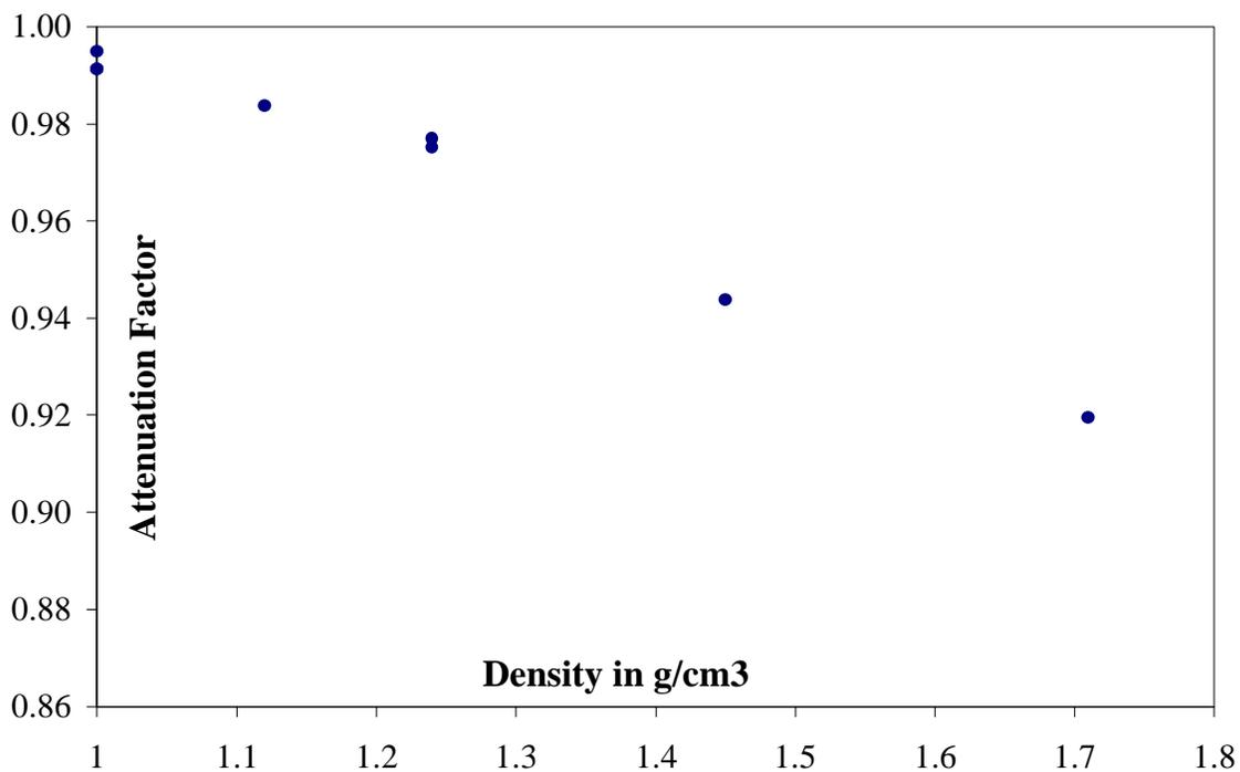
**Figure 5. Plot for the variation of attenuation factor of 185.7 keV as a function of density of solution (Cyl-2)**
