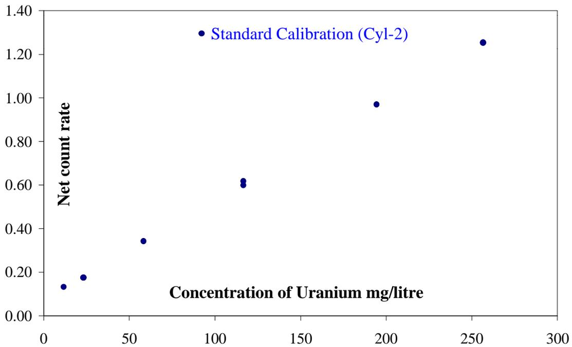
**Figure 4. Plot count rate for 185.7 keV of  $^{235}\text{U}$  as a function of amount of Uranium in the standard solution.**
