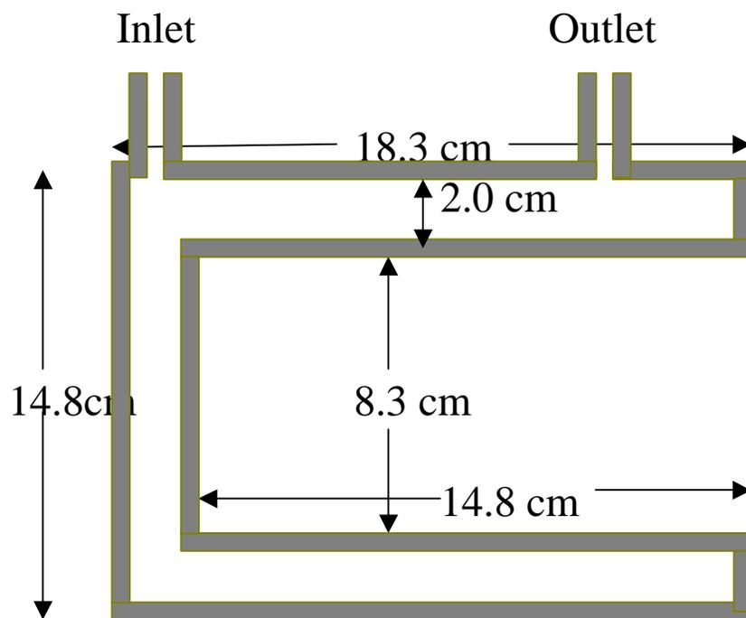
**Figure 1. Simulated container for the estimation of low concentration of uranium (mg/litre) in the solution stream.**
