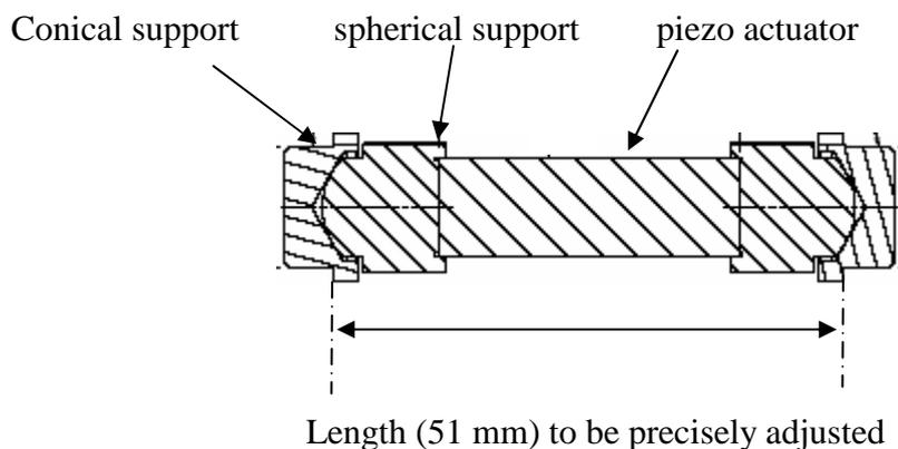
Figure 3: the sphere-cone system
