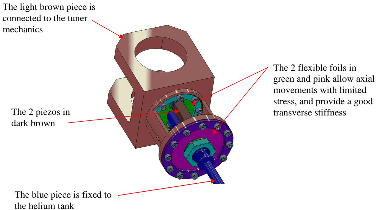
Figure 4: drawing of the piezos support
