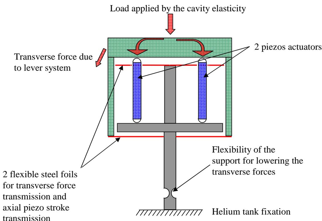
Figure 2: schematic view of the piezo actuators support.
