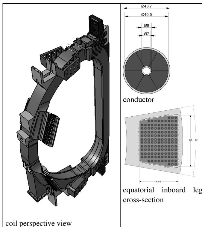
Fig. 1 : ITER TF coil design
