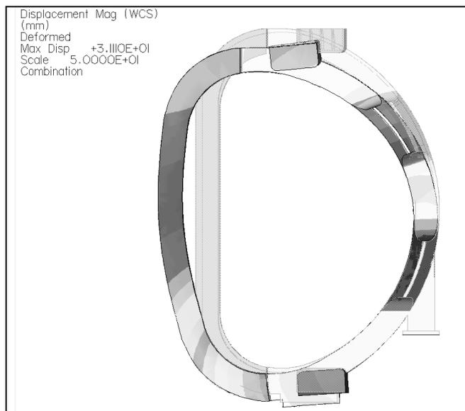
Fig. 2 : TF Coil deformation in a two-coil test at 34 kA
