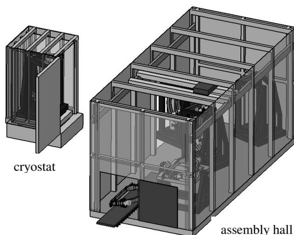
Fig. 3 : ITER TF Coil test facility outline design
