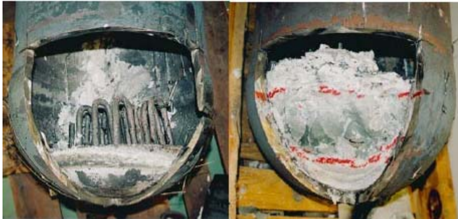
Figure 5. The in-vessel configurations of the FOREVER-EC4 test (left; failed vessel) and EC5 test (right; non-failed vessel).
