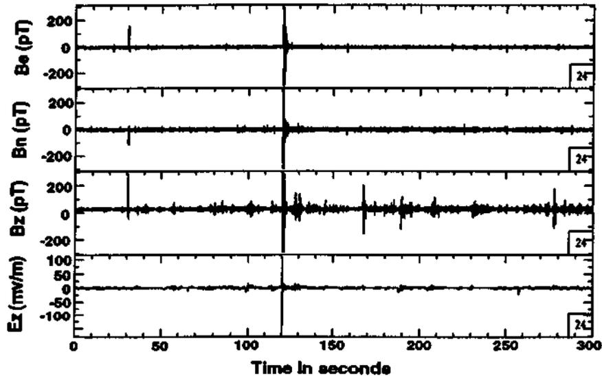
Figure 4. Low frequency EM data taken before and after detonation of Kuchen I. Detonation of the chemical explosive took place approximately at 120 s elapsed time. Note that the pulse occurring at approximately 30 s elapsed time is seen only in the magnetic components; it is related to the arming and firing signal. A fiducial reference timing pulse was not available during this phase of the experiment.
