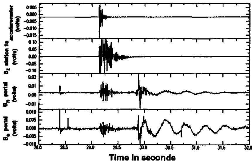
Figure 9. Signals recorded during the third Lynchburg mine explosion on April 12, 1996. The detonation time is not shown here, but the surface ground motion arrives at the 1a site first (top two traces, of the accelerometer and the magnetometer). As seen in Fig. 8, ground motion arrives about 0.04 seconds later at the portal. The large, low-frequency signal related to the air pulse arriving at the portal is again seen for this explosion.
