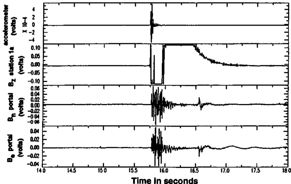
Figure 10. Signals recorded during the second Lynchburg mine explosion on April 4, 1996. The detonation time is not shown here, but the surface ground motion arrives at the 1a site first (top two traces, of the accelerometer and the magnetometer). As seen in Figs. 8 and 9, ground motion arrives about 0.04 seconds later at the portal. The smaller amplitude of the later air pulse in this figure is a scaling effect; the ground motion signals are much larger because of size of the detonation.
