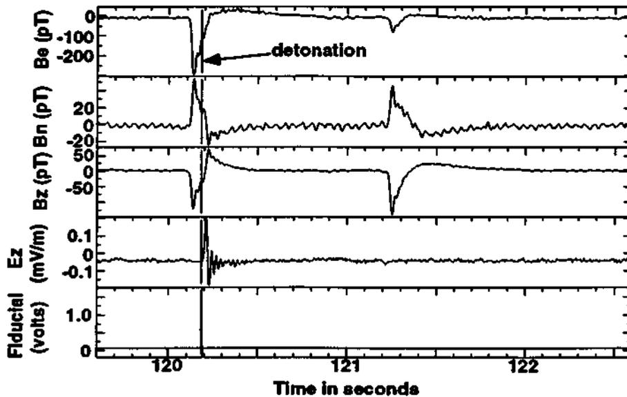
**Figure 3. Expanded view of pulses occurring at detonation time during the Kuchen III dry run. The fiducial pulse marks the detonation time (when firing pulse is sent to the bridgewires). No explosion took place during this part of the test, the firing signal was sent to a dummy load.**
