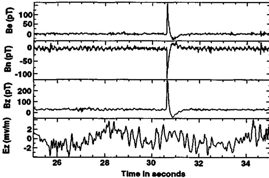
Figure 2. Expanded view of the pulse occurring 90 s before detonation during the Kuchen III dry run. No pulse is seen in the vertical electric component (bottom). The pulse seen on each of the three magnetic components is nearly identical to that seen 90 s before detonation for all three phases of Kuchen.
