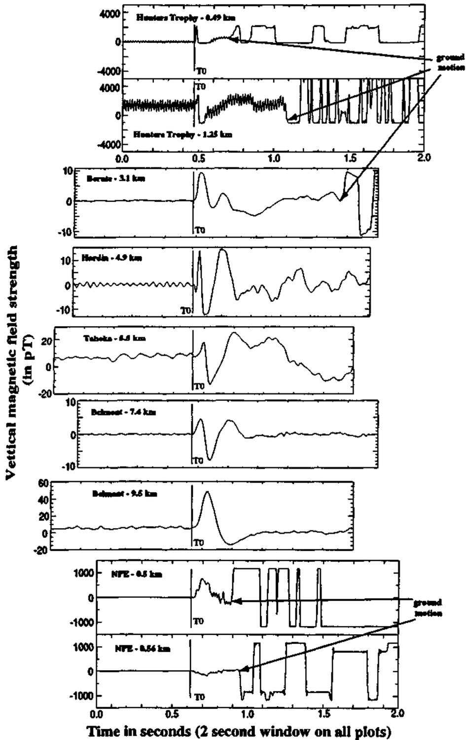
Figure 16. Vertical magnetic field data taken during six underground nuclear explosions (top seven traces) and one underground chemical explosion (bottom two traces). The name of each test and the slant range distance of the magnetometer are indicated. All traces show two seconds of data sampled at 100 to 200 Hz.
