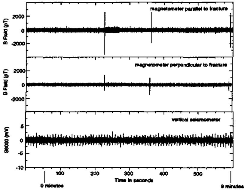
Figure 13. Magnetic (upper two traces) and seismic (bottom trace) signals recorded during the hydrofrac experiment at Lost Hills at site 1. Times in minutes at the bottom of the figure correspond to times shown in Fig. 12.
