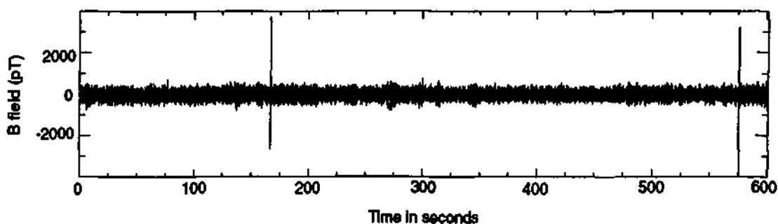
**Figure 15. Magnetic field signal recorded at site 2 three hours before the start of the hydrofrac operation. Signal spikes similar to those seen in Fig. 13 and Fig. 14 are also seen here and are probably power system noise.**
