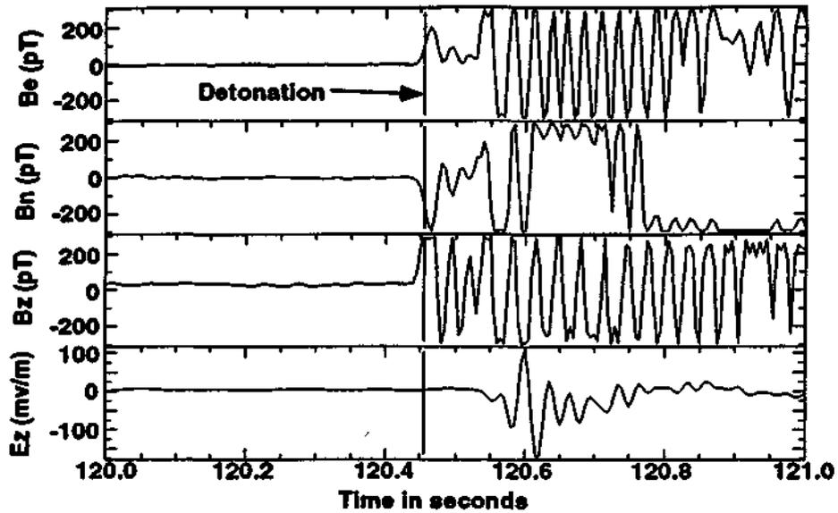
Figure 5. Low frequency EM signals near detonation time during Kuchen I. Detonation time (0600:00.072 PDT) is indicated by the vertical bar. Note that the first signal arrival precedes the detonation time in the magnetic components, similar to what was seen during the dry run (Fig. 3). A second pulse, seen on the east and north magnetic components, just when the electric signal starts and arriving about 70 ms after detonation, is due to ground motion arriving at the sensors.
