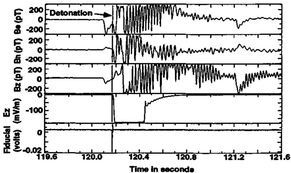
Figure 6. Low frequency EM data taken during the Kuchen II underground chemical explosion. Detonation time (see text) is indicated by a vertical bar. For this part of the test series, a fiducial signal was available to record the detonation time.
