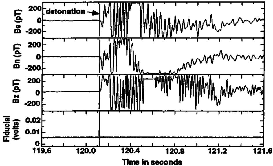
Figure 7. Low frequency EM data taken during the Kuchen III underground chemical explosion. Detonation time (see text) is indicated by a vertical bar and by the fiducial signal. The vertical electric channel for this test was inoperative.
