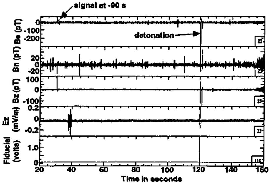
Figure 1. Signals recorded during the dry run for Kuchen Phase III, on August 30, 1995. A pulse is seen 90 s before detonation time in the three magnetic channels, but not on the vertical electric channel. A larger pulse is seen at detonation time on all three magnetic channels and on the vertical electric. The fiducial pulse gives a reference for the detonation time.
