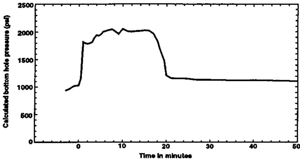
**Figure 12.** Pressure at the bottom of the borehole (calculation based on measured surface pressure and length of hydrostatic column in the well) during the last phase of the hydrofracture. The fracture is initiated during the initial rapid rise in pressure. Fracture extension occurs during the 20 minutes when the pressure varies between 1800 and 2100 psf.
