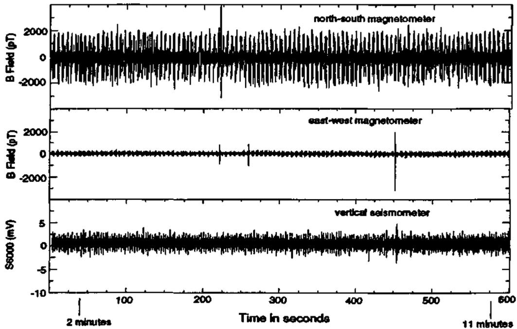
Figure 14. Magnetic (upper two traces) and seismic (bottom trace) signals recorded during the Lost Hills hydrofrac experiment at site 2. Times in minutes at the bottom of the figure correspond to times shown in Fig. 12.
