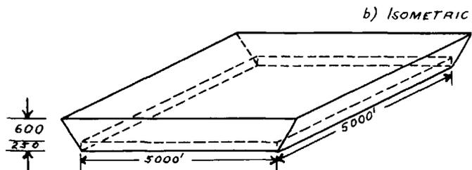
FIGURE 1: THE OREBODY AND ITS OVERBURDEN
