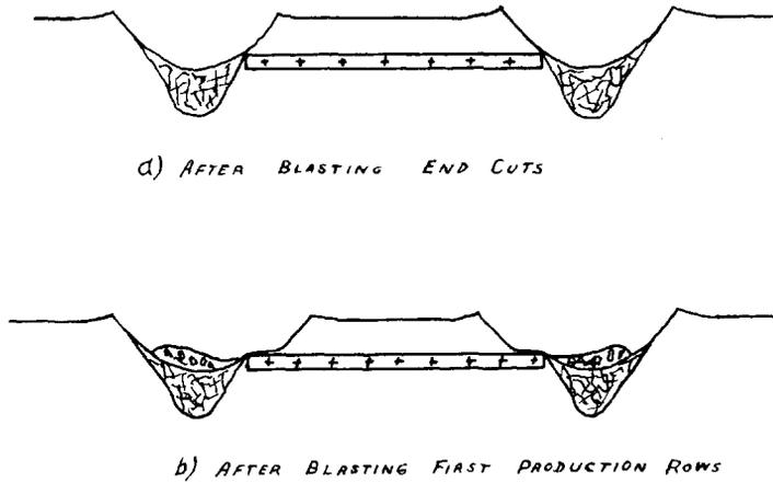
FIGURE 6: DOUBLE-CUT METHOD
