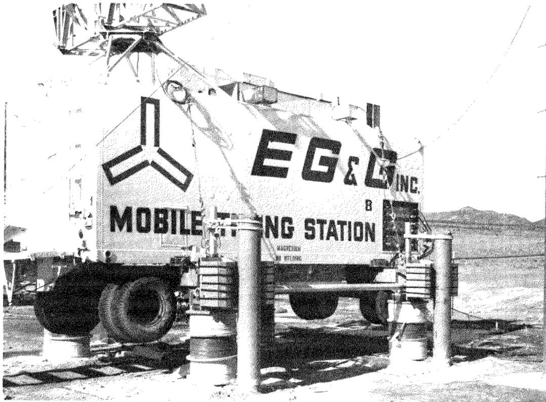
Fig. 8. Post-shot photo of trailer on U. G. C. system with horizontal alignment control.
