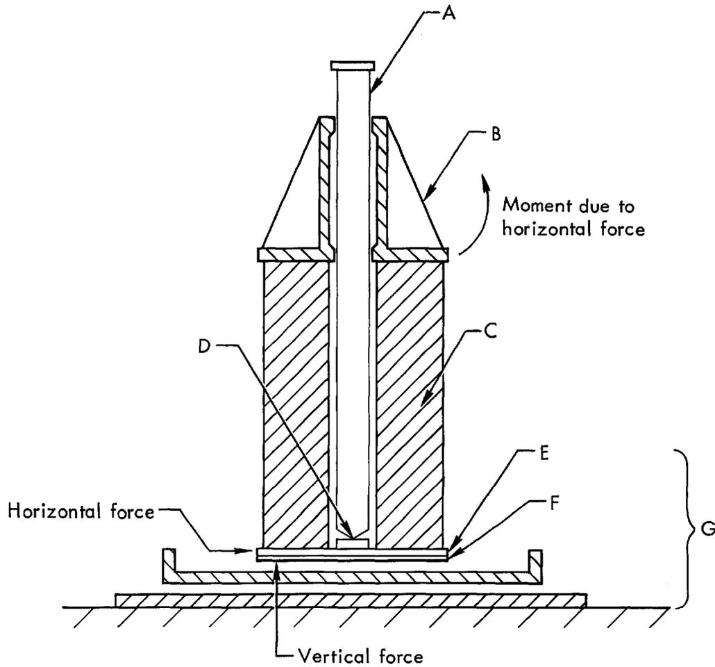
Fig. 7. U.G.C. characteristics: (A) Column, (B) crossbeam, (C) crushable material, (D) pivot joint, (E) metal disc, (F) Teflon, (G) anti-friction surface pad, exploded for clarity.
