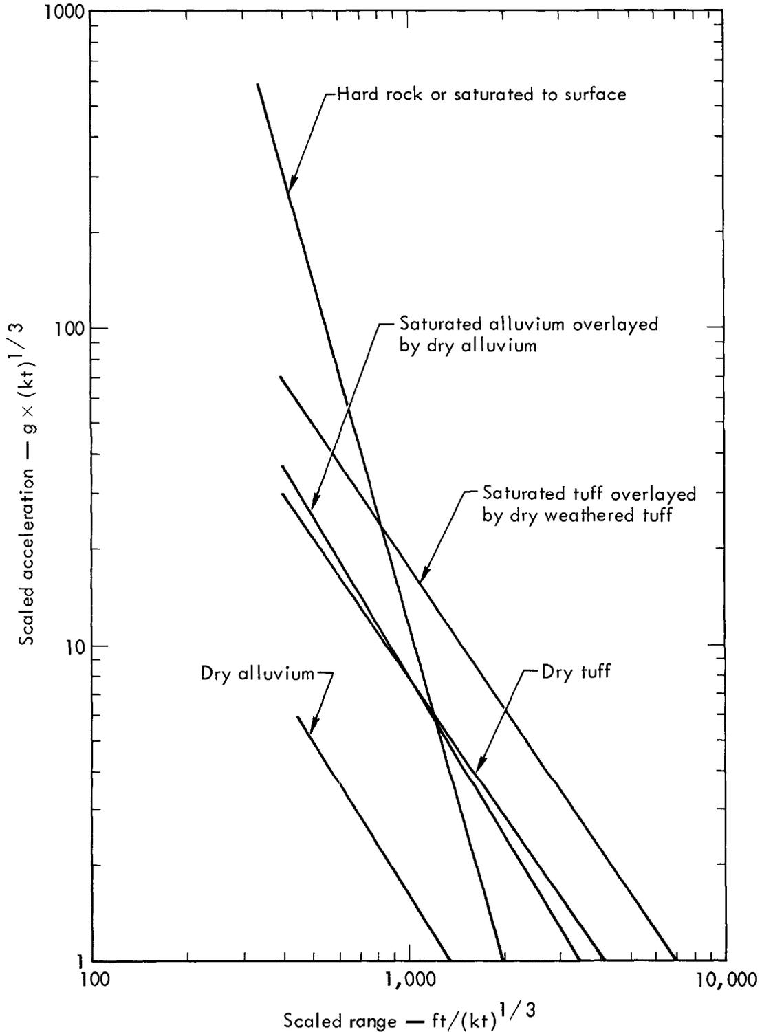
Fig. 3. Scaled initial peak-particle accelerations for various geologies. Note: Surface values for acceleration are material-limited for geologies with a weathered surface layer. This fact is obscured by the acceleration scaling.
