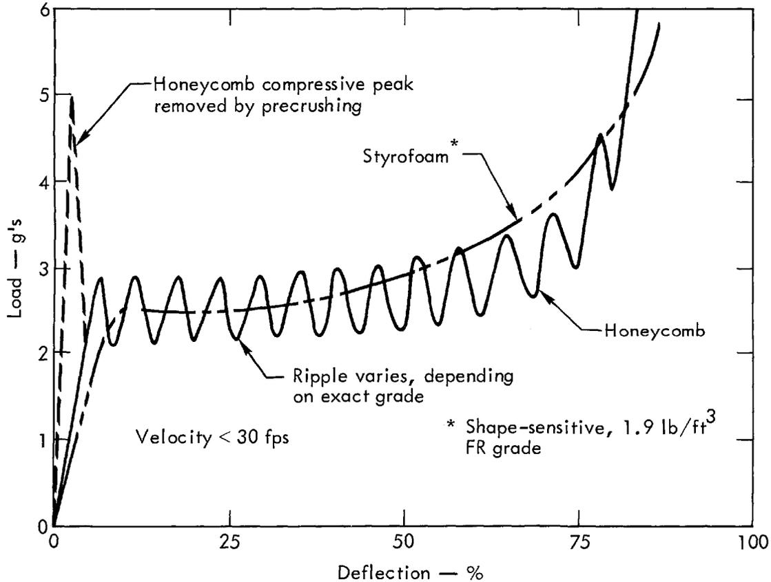
Fig. 10. Typical dynamic load-deflection curve for a honeycomb and a styrofoam material.
