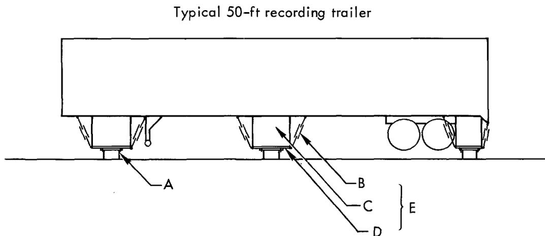
Fig. 11. F&RC shock-mitigation system: (A) Replaceable foam pad bolted to cribbing, (B) turnbuckle tie, (C) wood cribbing with plywood scabbing, (D) angle iron frame, (E) reusable cribbing assembly.
