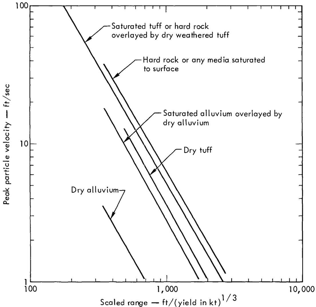
Fig. 1. Peak particle surface velocities for various geologies.
