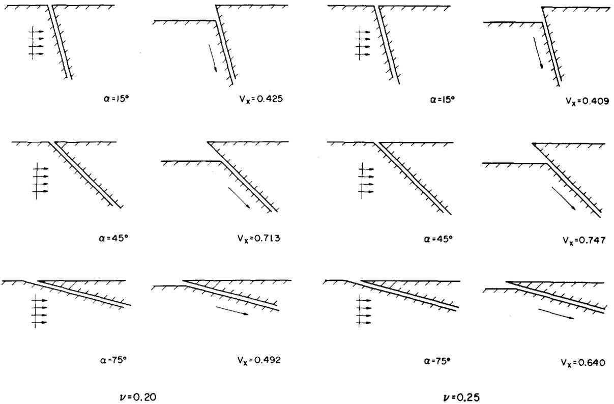
Fig. 9. Surface displacements caused by a square topped transient stress wave impinging against a loose fracture or fault.  $\nu = 0.20$ .
