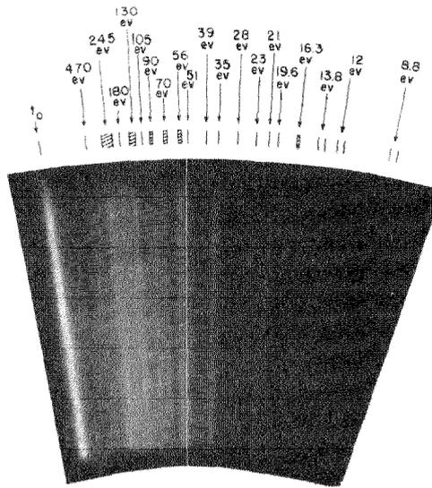
Fig. 1. Autoradiograph of  $^{235}\text{U}$  wheel, 1958 experiment.
