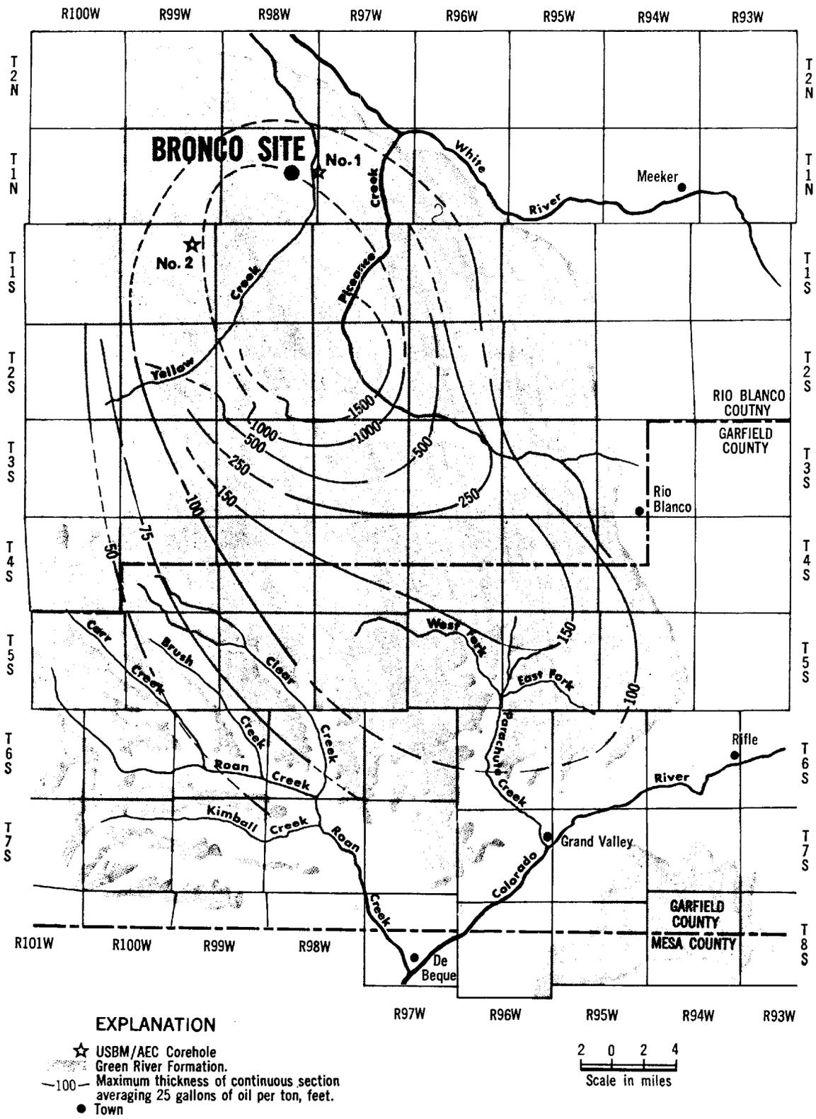
Fig. 2. Isopachous map of 25 gal/ton oil shale, Piceance Creek Basin, Colorado.
