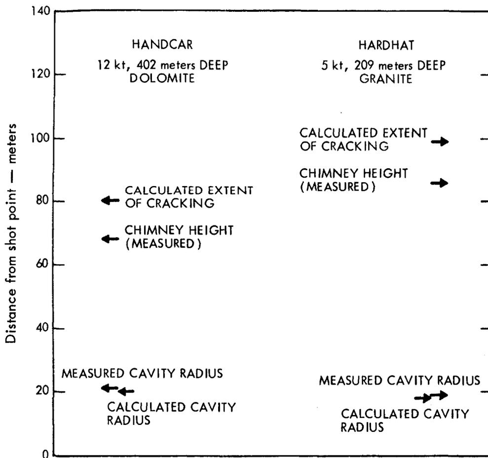
Fig. 4. Calculated cavity radii for Handcar and Hardhat, compared with observed dimensions.<sup>12</sup>
