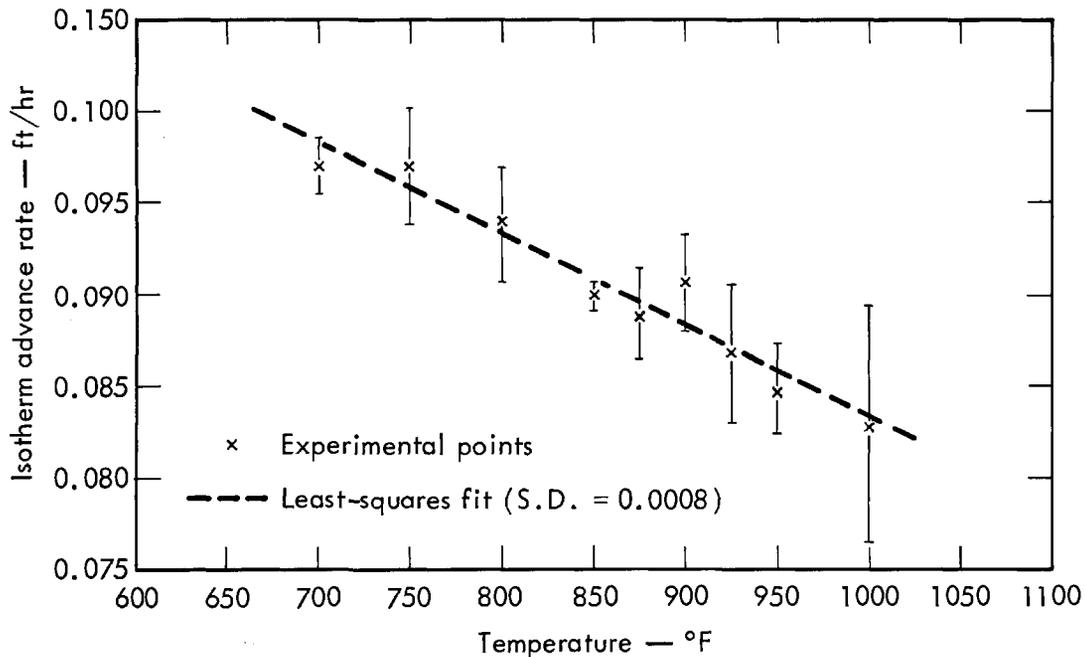
Fig. 8. Isotherm advance rates: Average of Laramie 10-ton retort runs 8, 9, 10, 11.
