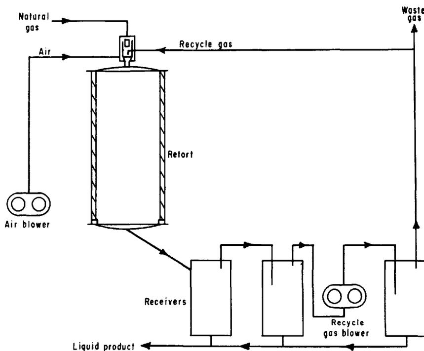
Fig. 7. Schematic diagram of the 150-ton retort.
