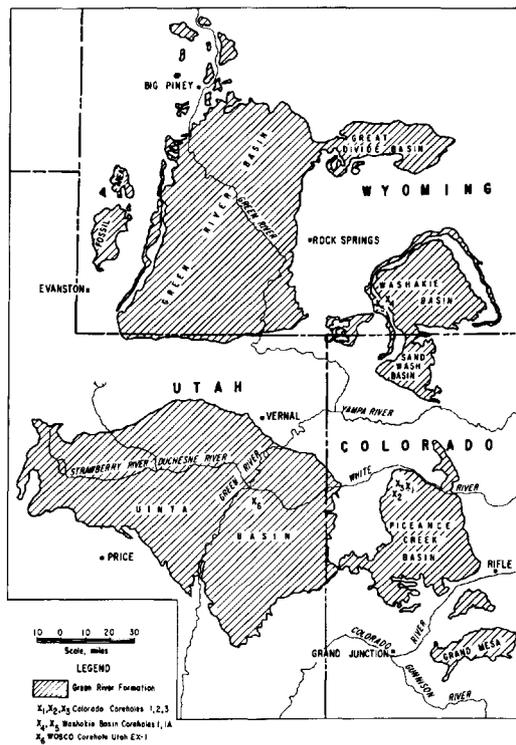
FIGURE 1. - Coreholes in the Green River Formation investigated for nuclear fracturing.
