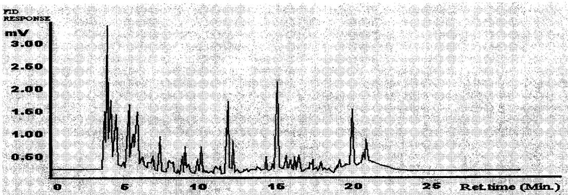
Fig. 1 (a) Pyrogram of Algae (*Chlorella kessleri*) obtained by Py-GC analysis
