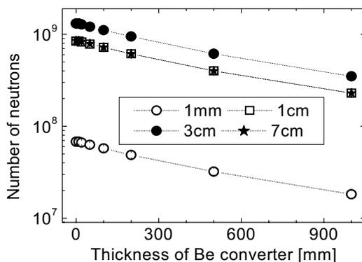
**Fig. 2** Neutron production by the  $10^{14}$  electron beam with energy 15 MeV in beryllium converter after 1 mm, 1 cm, 3 cm and 7 cm of tungsten converter. Neutron production for 1 cm and 7 cm tungsten layer is almost the same.
