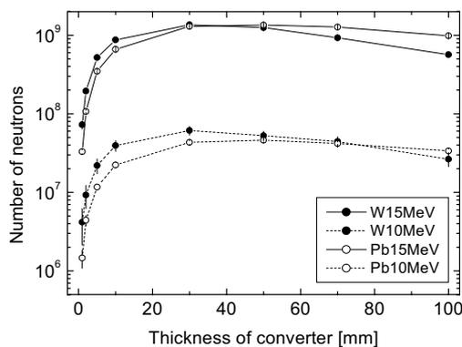
**Fig. 1** Number of neutron detected behind the tungsten and lead converters bombarded by  $10^{14}$  monoenergetic 10 MeV and 15 MeV electrons.
