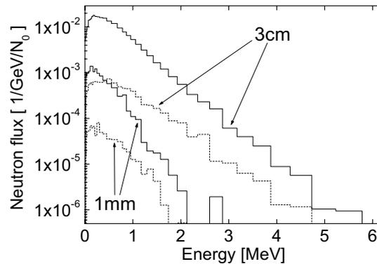
**Fig. 3** Energy spectra of produced neutrons for 10 MeV and 15 MeV electron beam for two arbitrarily chosen tungsten converter thickness (1 mm and optimal for neutron yield 3 cm).
