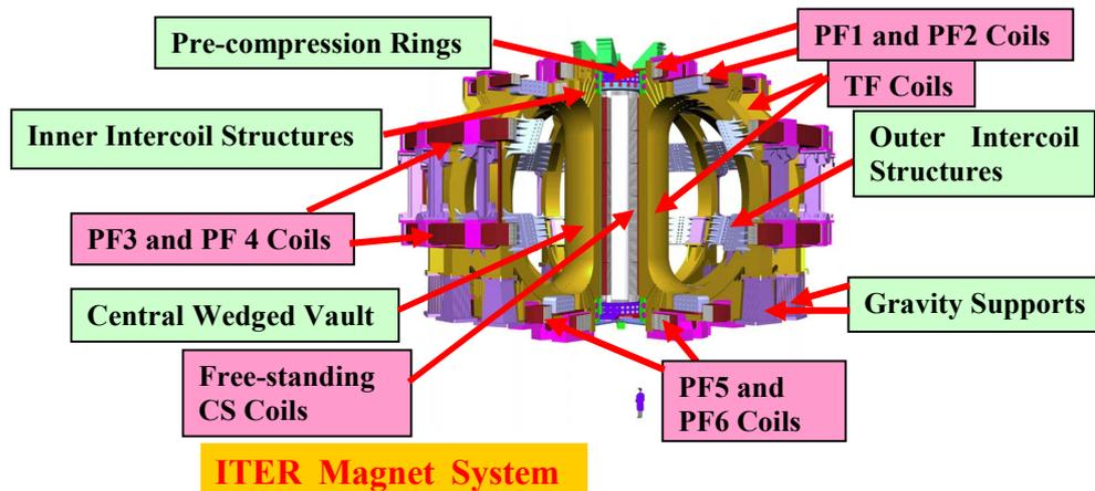
Figure 2: The ITER magnet system showing the toroidal field (TF) coils, the poloidal field (PF) coils, the central solenoid (CS) and associated structural features.
