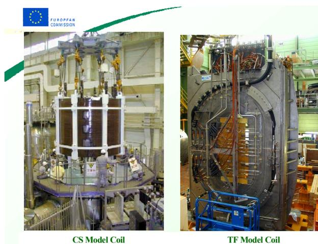
Figure 3: (left) The CS Model Coil is shown being installed in a cryostat prior to testing at Naka, Japan. (right) The TF Model Coil is shown being prepared for its testing in a cryostat at the Forschungszentrum Karlsruhe (Association EURATOM/FZK), Germany.
