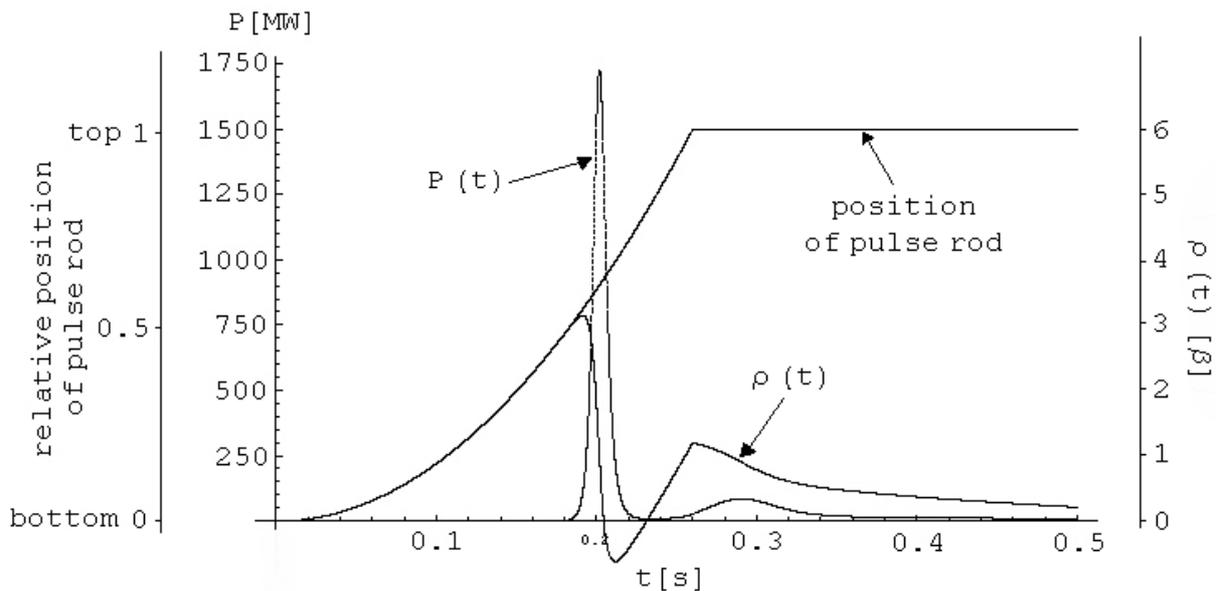
Figure 3.4: Power, pulse rod position and reactivity of the system for inserted reactivity  $6\beta$
