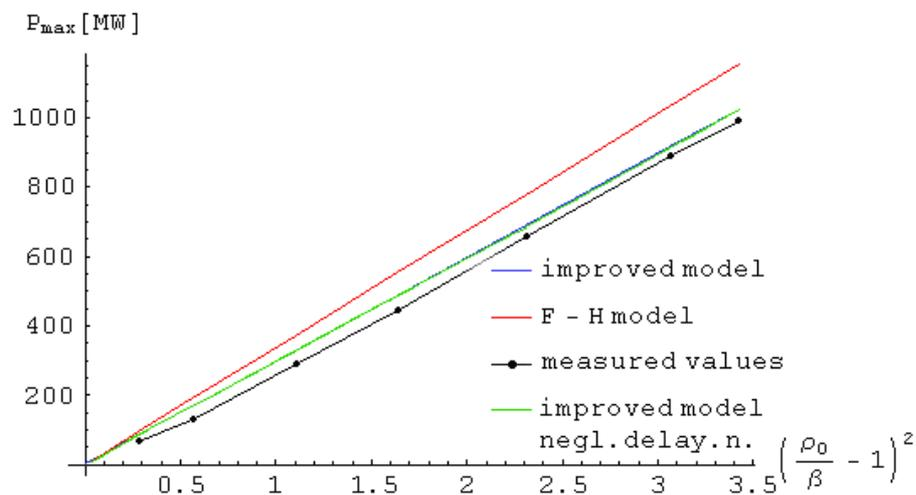
Figure 2.2 b): Comparison between measured values of maximal power in the pulse and values calculated by F-H model, improved model and model that neglects delayed neutrons.
