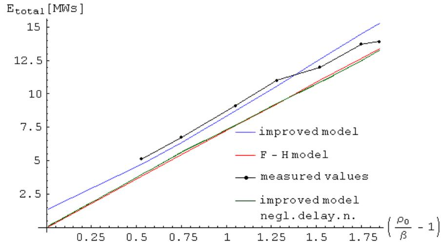
Figure 2.2 a): Comparison between measured values of total released energy in the pulse and values calculated by F-H model, improved model and model that neglects delayed neutrons.
