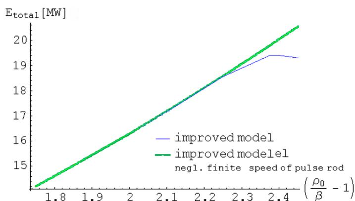
Figure 2.4 a): Comparison of total released energy in the pulse calculated with improved model and model that neglects contributions of finite speed of pulse rod
