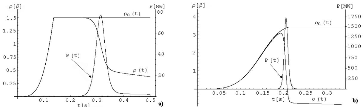
Figure 2.5: Time dependence of power, inserted reactivity and reactivity of the system for small a) and high b) inserted reactivity calculated by *improved model*
