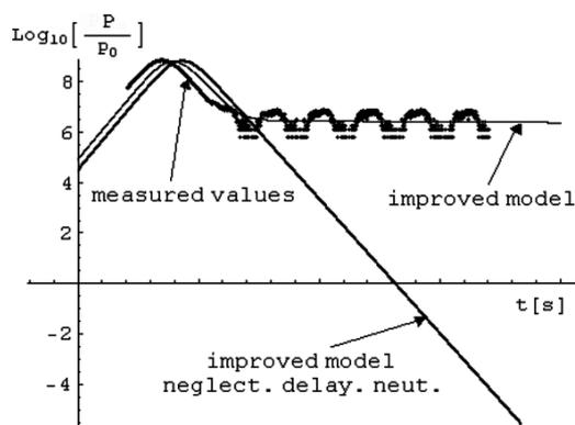
Figure 2.3: Power as a function of time for measured values, improved model and model that neglects delayed neutrons
