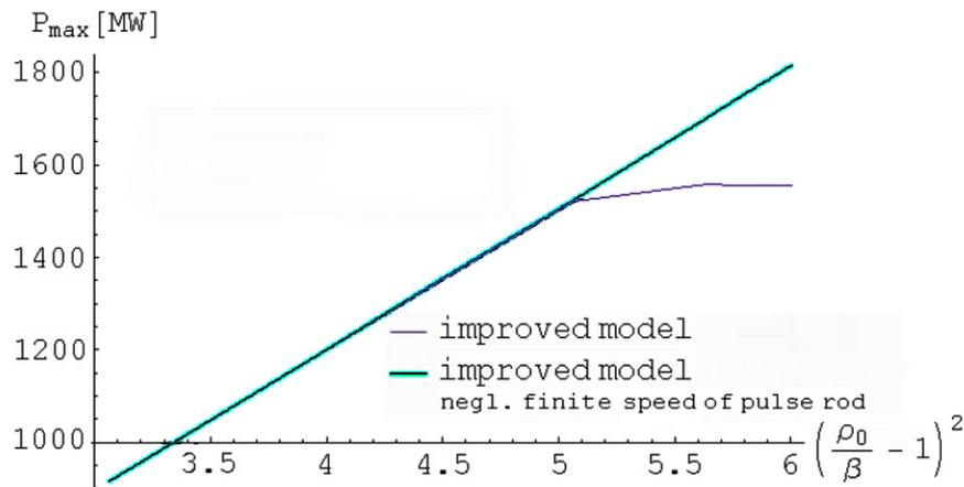
Figure 2.4 b): Comparison of maximal power in the pulse calculated with improved model and model that neglects contributions of finite speed of pulse rod
