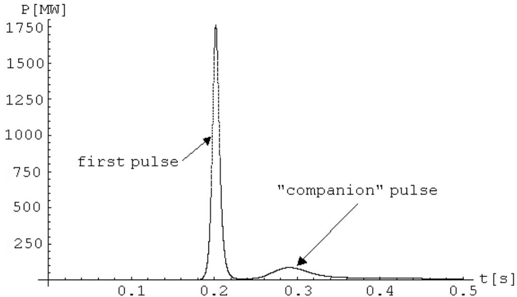
Figure 3.1: Power course predicted by improved model for inserted reactivity  $6\beta$
