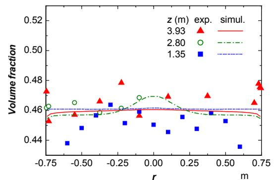
Figure 4. Steady state 1: experimental and simulated radial profiles of steam volume fraction.
