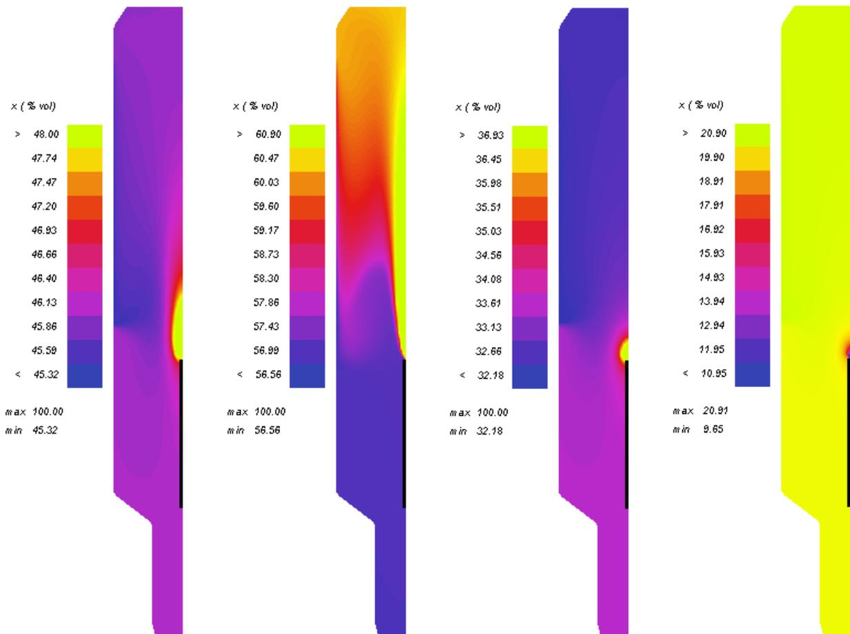
Figure 13. Steady state 1: steam volumetric concentration.
