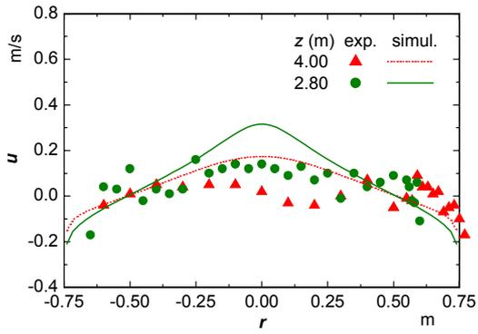
Figure 5. Steady state 1: experimental and simulated radial profiles of vertical velocity.
