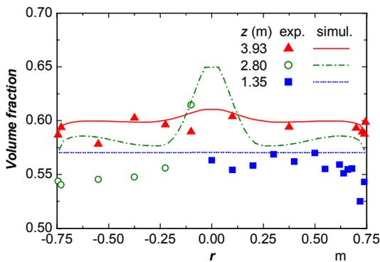
Figure 7. Steady state 2: experimental and simulated radial profiles of steam volume fraction.
