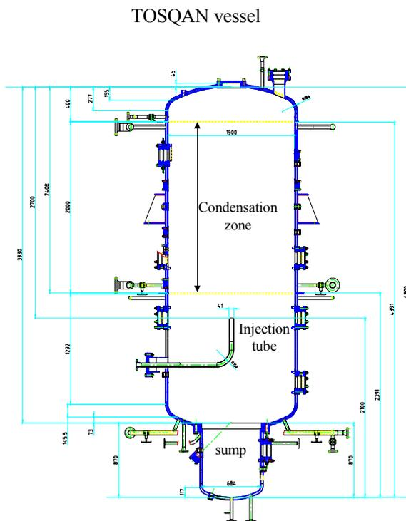
Figure 1. Schematic view of the TOSQAN experimental facility [7].
