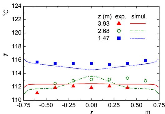
Figure 3. Steady state 1: experimental and simulated temperature radial profiles.
