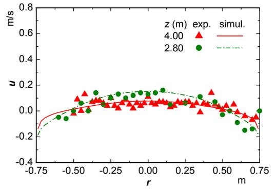
Figure 12. Steady state 3: experimental and simulated radial profiles of vertical velocity.
