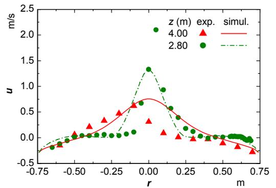
Figure 8. Steady state 2: experimental and simulated radial profiles of vertical velocity.
