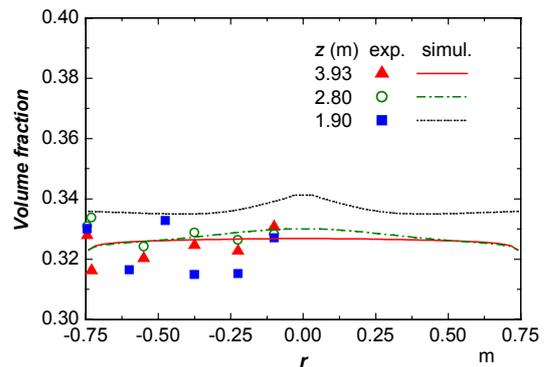
Figure 10. Steady state 3: experimental and simulated radial profiles of steam volume fraction.
