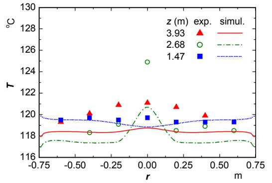
Figure 6. Steady state 2: experimental and simulated temperature radial profiles.
