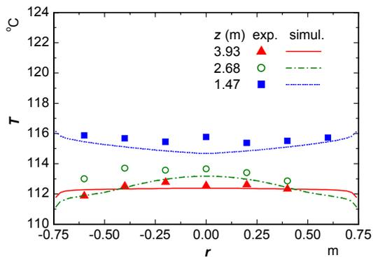
Figure 9. Steady state 3: experimental and simulated temperature radial profiles.
