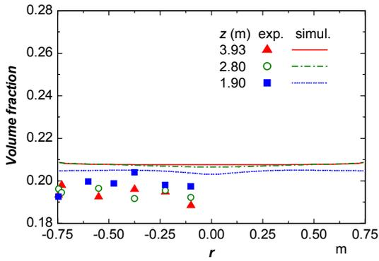
Figure 11. Steady state 3: experimental and simulated radial profiles of helium volume fraction.
