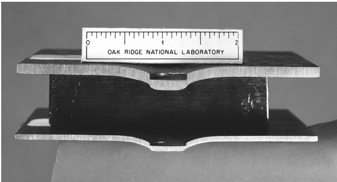
Fig. 2. Cross sections of steel test plates that were not punctured
