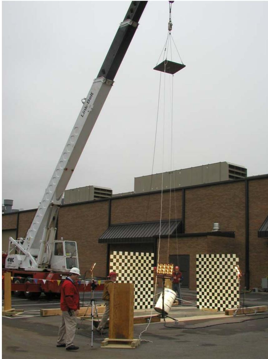
**Figure 2. Crush Test of ES-2100 at NTRC (December 2002)**
