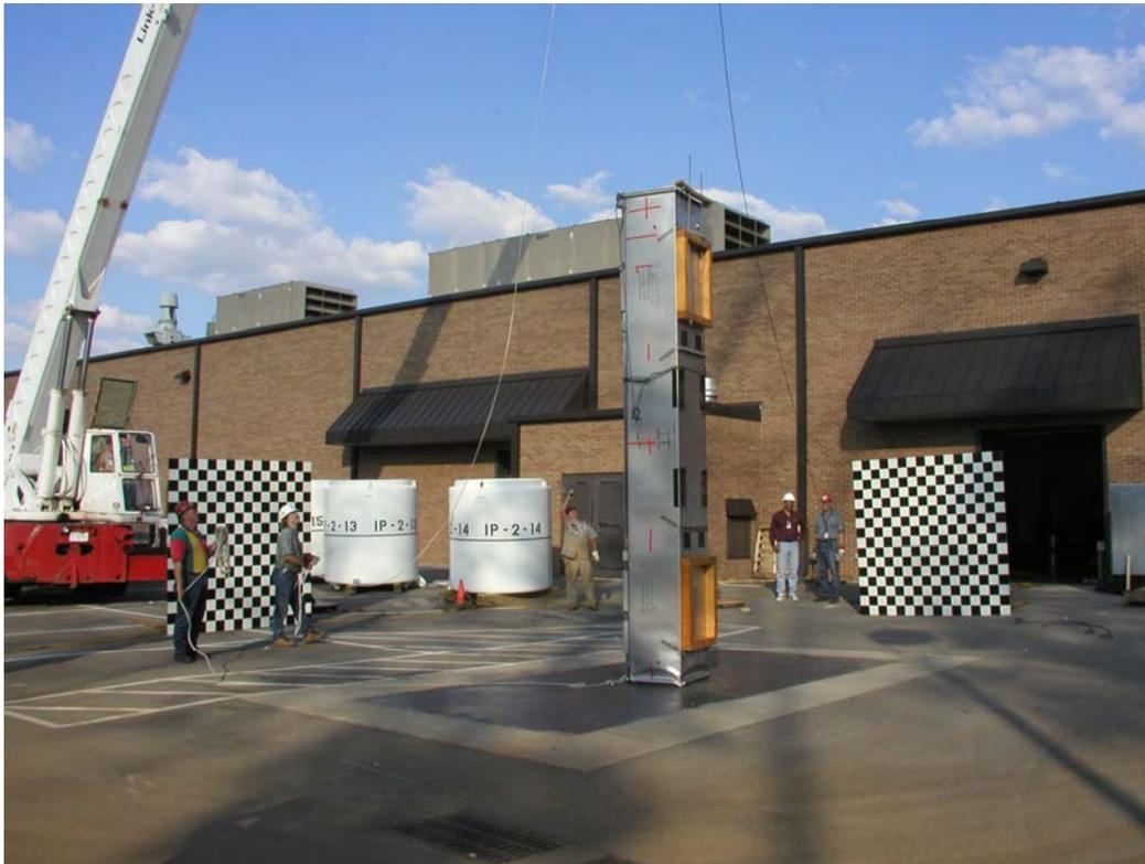
Figure 7. 9-m Drop Test of the RAJ-II BWR Fresh Fuel Package (Perfect Drop)
