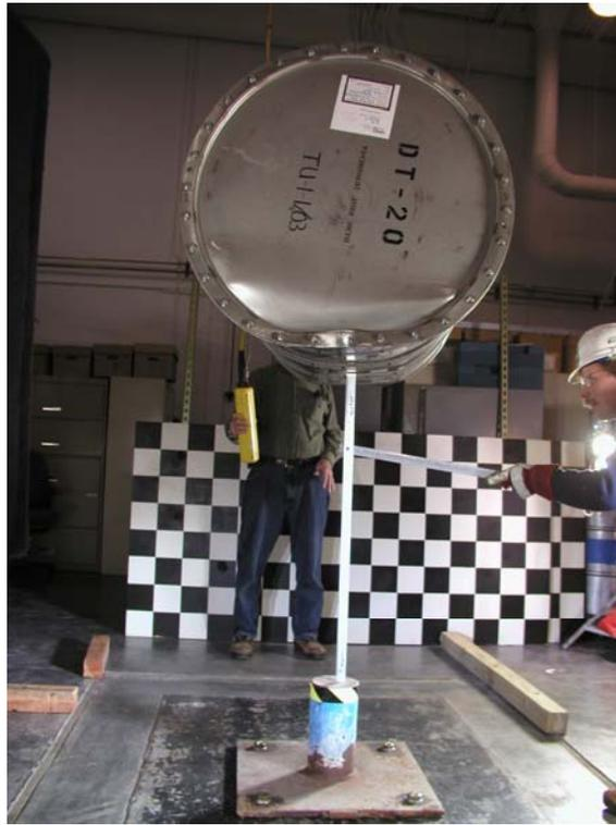
**Figure 3. Puncture Test Preparation of the DT-20 Inside the PRF**
