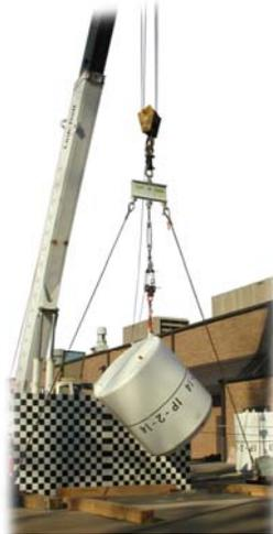
Figure 6. Corner Drop of the Fernald Silo IP-2 Waste Package at NTRC
