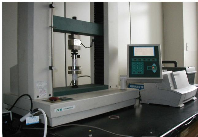
Fig. 1. Compression Tester (Hounsfield, H25K-ST)
