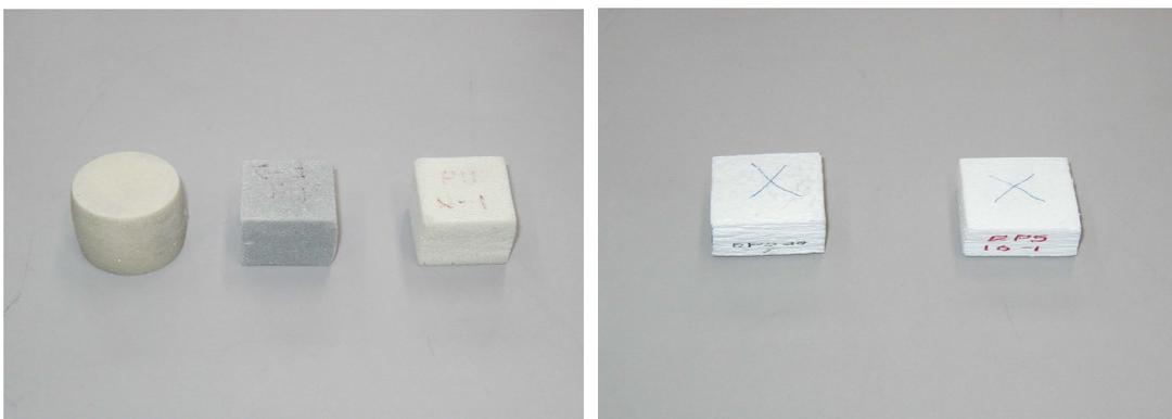
Fig. 2. Specimen of Polyurethane Foam and Styrofoam
