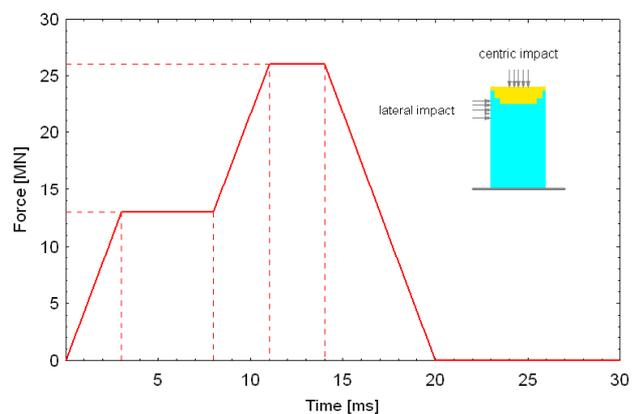
Fig. 1: Load vs. time function for the MEPPEN test projectile described in [9]
