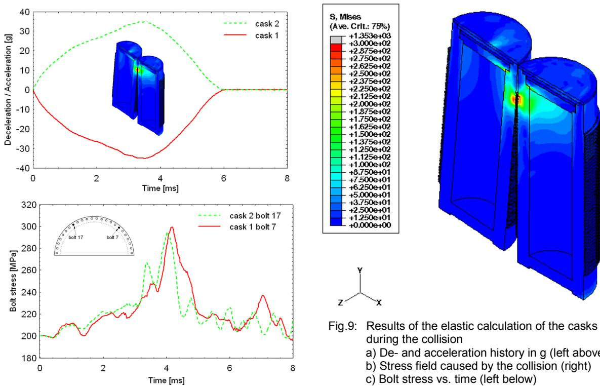
Fig.9: Results of the elastic calculation of the casks during the collision
