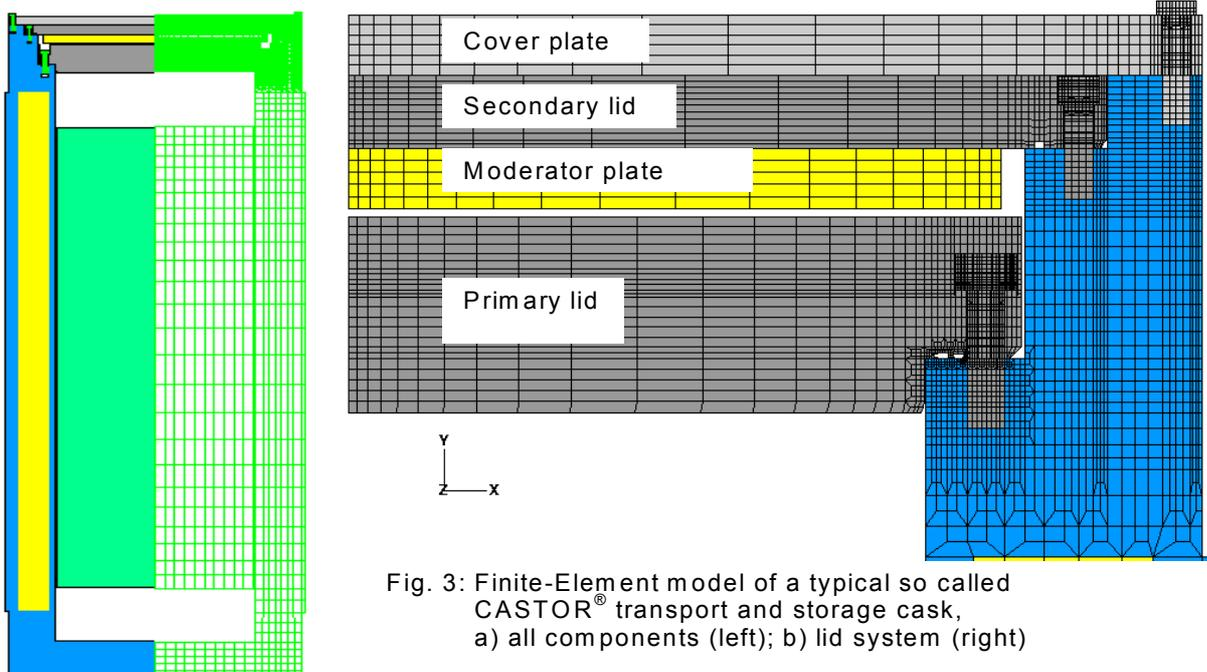
Fig. 3: Finite-Element model of a typical so called CASTOR<sup>®</sup> transport and storage cask, a) all components (left); b) lid system (right)
