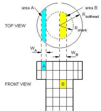
Fig. 2: Cross-sectional views of the bolt head and the shank [11]
