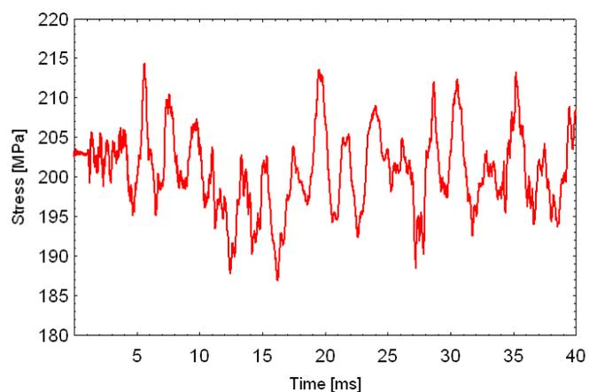
Fig. 5: Time dependence of the tensile stress component in the primary lid bolts
