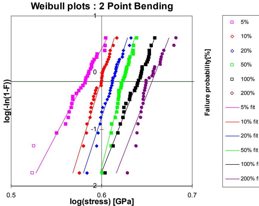
Evolution of the mechanical strength as a function of the applied stress rate, after irradiation up to MGy dose levels.
